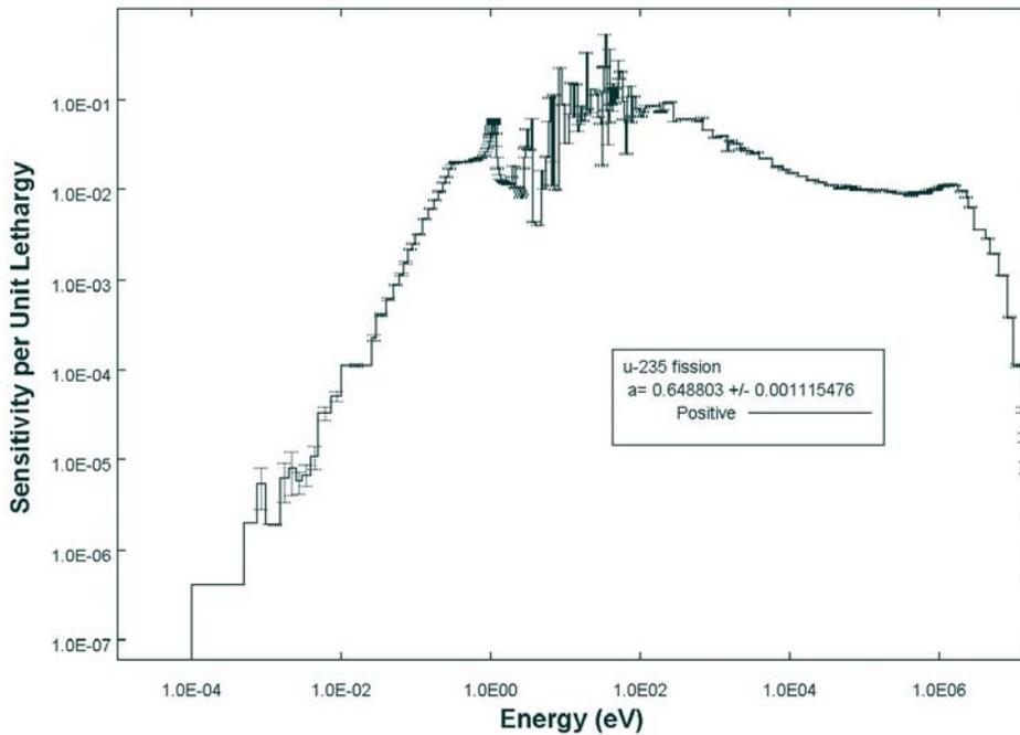
**Fig. 3** Sensitivity of  $k_{eff}$  to the  $^{235}\text{U}$  fission cross section for the HISS/HUG benchmark.
