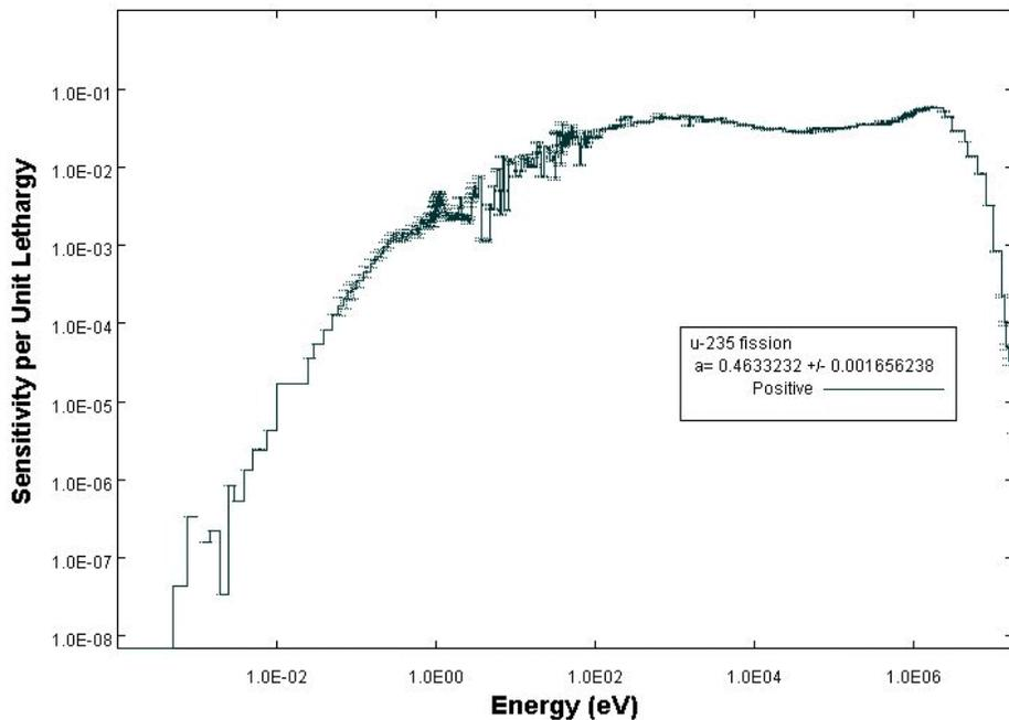
neutron group structure of the SCALE system.<sup>11)</sup> Figures 2 and 3 show that a component of the  $k_{eff}$  is due to the unresolved energy region.
