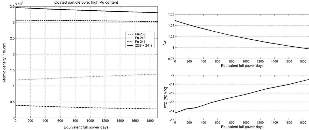
**Fig 7:** Coated particle core, high Pu content. Left: atomic density of 3 Pu isotopes, atomic density of fissile material (Pu-239 and Pu-241). The total atomic density of fissile material at EOC is smaller than at BOC, even though the density of Pu-239 is almost constant. Right:  $k_{eff}$  and FTC during burnup. At the end of the irradiation  $k_{eff}$  is 0.98.
