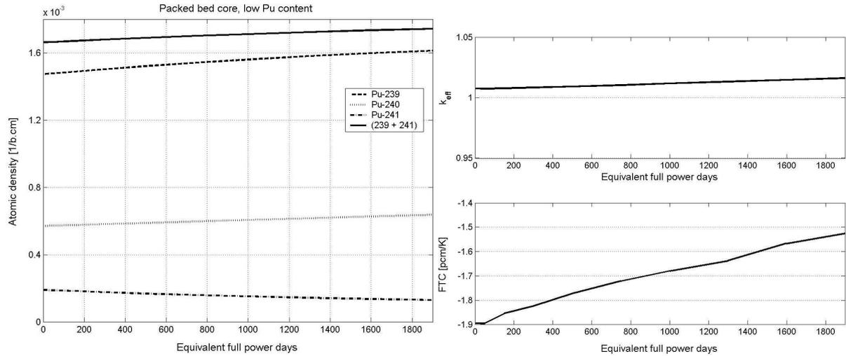
**Fig 4:** Hollow fuel sphere core, low Pu content. Left: atomic density of 3 Pu isotopes, atomic density of fissile material (Pu-239 and Pu-241). The total atomic density of fissile material at EOC is larger than at BOC. Right:  $k_{eff}$  and FTC during burnup. Note the increase in  $k_{eff}$  with burnup.
