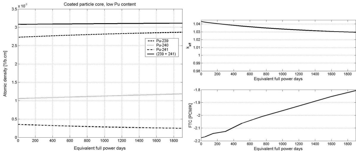
**Fig 6:** Coated particle core, low Pu content. Left: atomic density of 3 Pu isotopes, atomic density of fissile material (Pu-239 and Pu-241). The total atomic density of fissile material at EOC is slightly larger than at BOC, but the increase is very small. Right:  $k_{eff}$  and FTC during burnup. The initial value of  $k_{eff}$  is larger than 1.04, so the Pu content can be reduced further to improve conversion.
