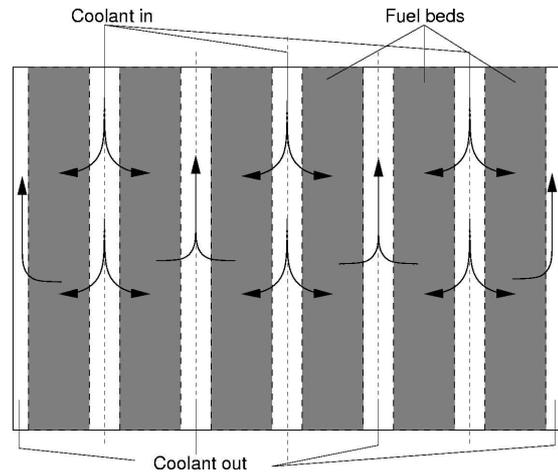
**Fig 2:** General layout for a GCFR core using hollow fuel spheres (axial cross section through cylindrical core, not to scale). The coolant enters from the top, flows radially through the beds and exits again at the top.
