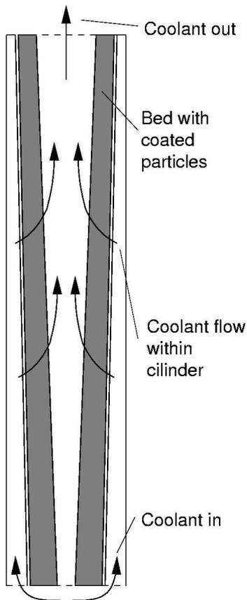
**Fig. 3:** Cross section of an annular cylinder with a fuel bed of CPs (not to scale).
