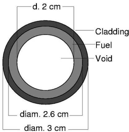
**Fig 1:** a hollow fuel sphere. The central void is empty to accommodate fission gas release and fuel swelling.
