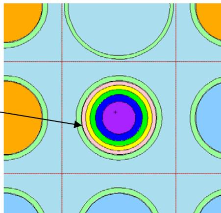
**Figure3a:** Quarter of GEDEON cluster with 24 depleting mediums
