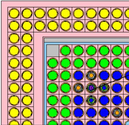
**Figure3b:** Five depleting mediums for the UOX-Gadolinium rod (+) and the burnup tracer rods
