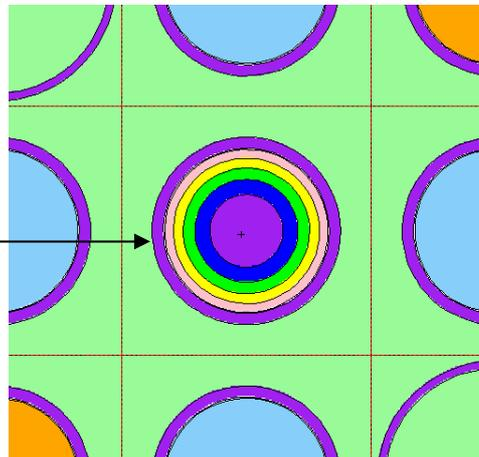
**Figure 2a:** Quarter of MOX assembly with 8 depleting mediums
