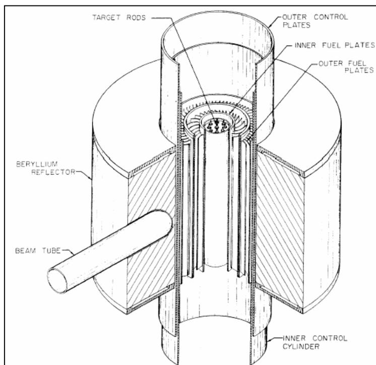
Fig. 1 Configuration of HFIR core and control elements
