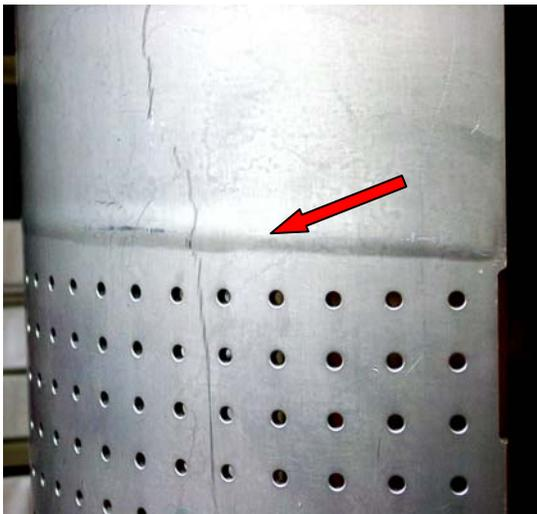
**Fig. 2** Blister at tantalum/europium interface of a safety plate.
