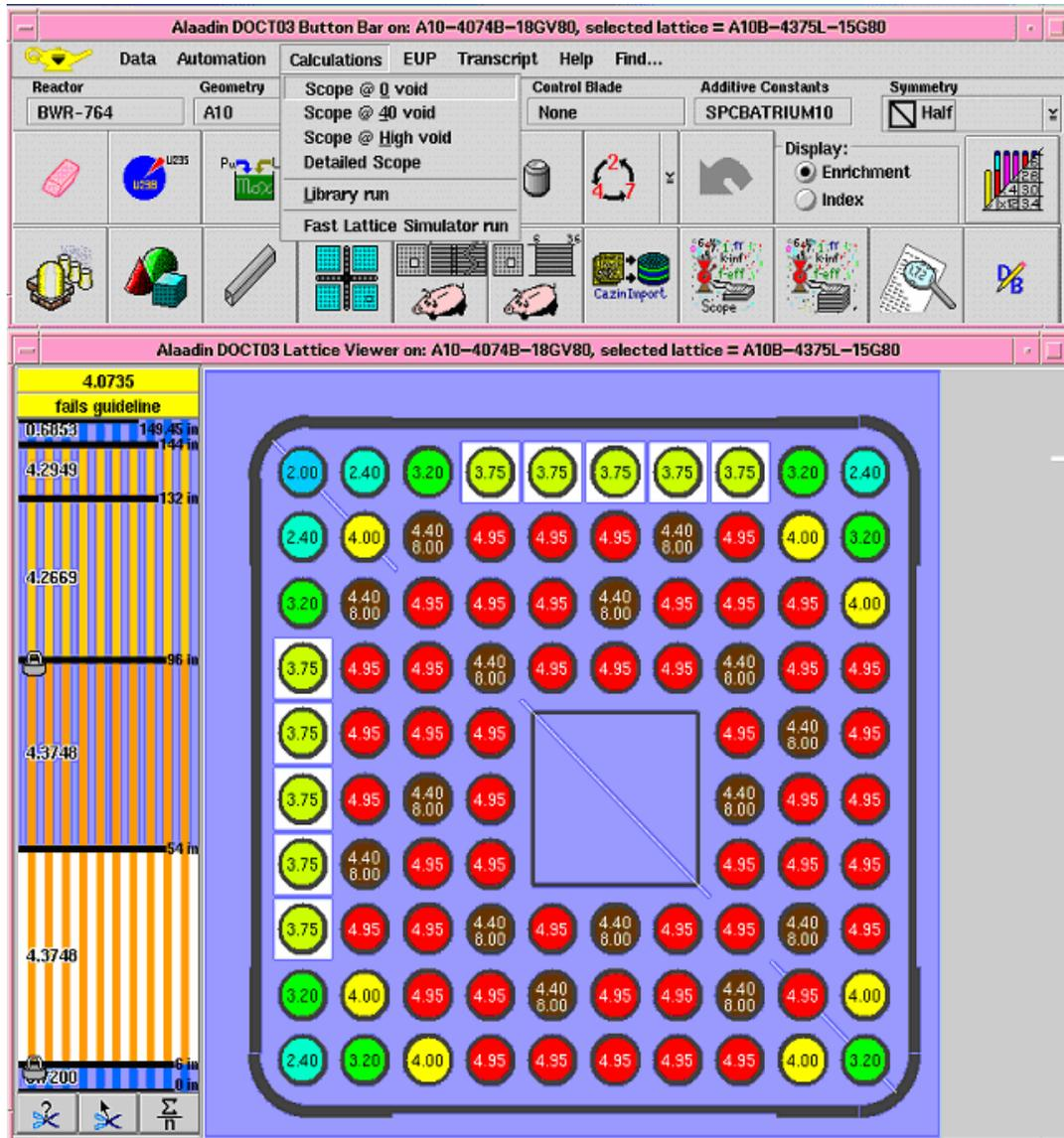
Figure 1 ALAADIN Standard Menu Bar And A Typical Lattice View
