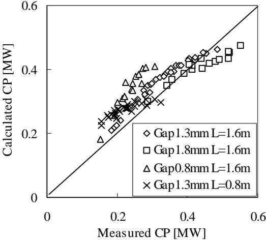
**Fig.8** Measured critical power versus calculated critical power with Arai's correlation
