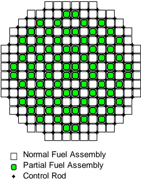
**Fig.1** BARS core layout
