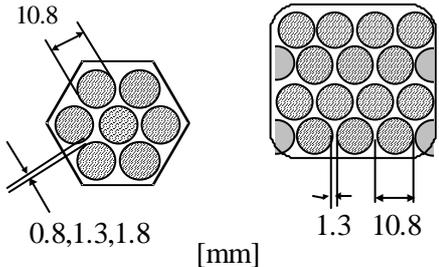
**Fig.7** Cross-sectional view of test assemblies
