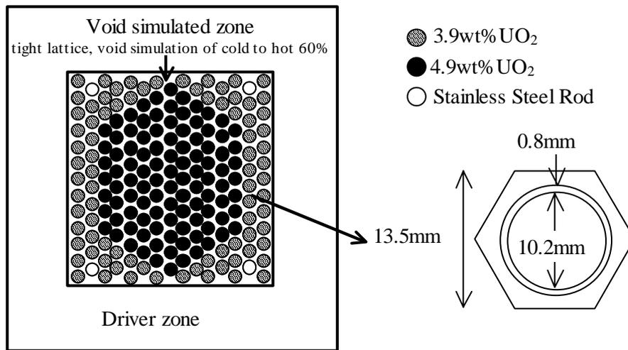
**Fig.3** Experimental core configuration for critical assembly test
