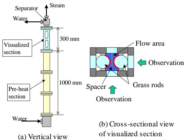
**Fig.5** Schematic view of visualized test section
