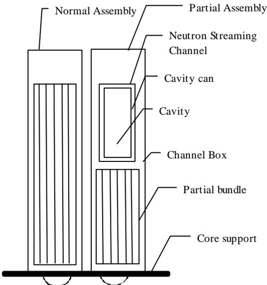
**Fig.2** Vertical View of Fuel Assembly
