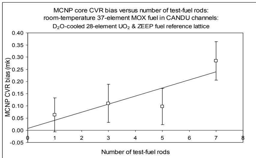
**Fig. 3** MCNP core CVR bias versus number of test-fuel rods
