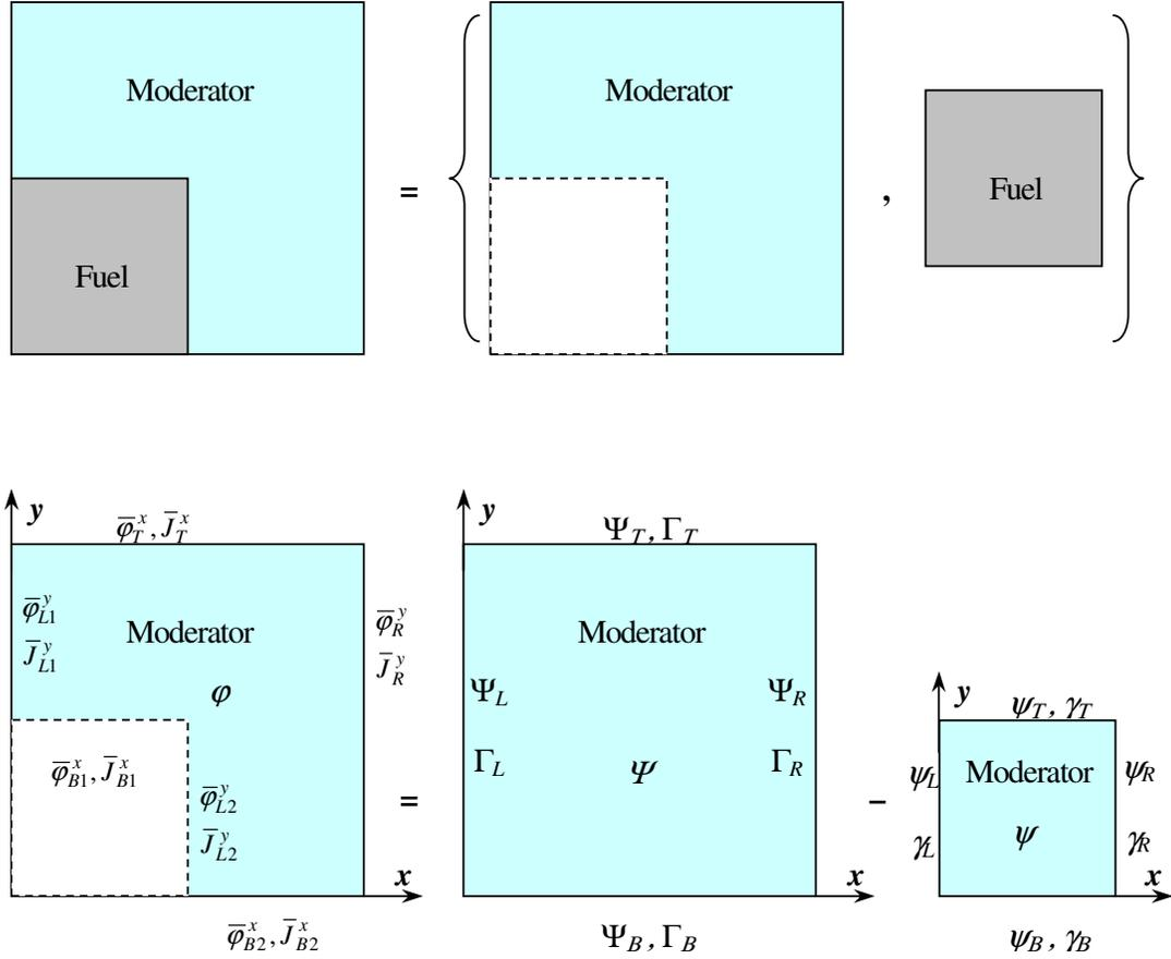
**Fig.1** Cartesian-geometry approximation of the unit cell configuration (top), and representation of the moderator CC as the difference between two cc's (bottom).
