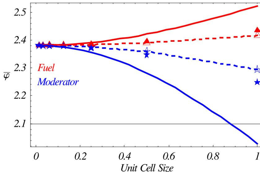
**Fig. 2** Fuel- and moderator-averaged scalar fluxes vs unit-cell size as computed by the new method (solid lines), the FD method converged with mesh refinement (dashed lines), and the FD method on a  $2 \times 2$  mesh (solid symbols).
