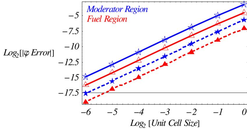
**Fig. 3** Error in the fuel- and moderator-averaged scalar fluxes vs unit-cell size as computed by the new method (solid lines) and the FD method on a  $2 \times 2$  mesh (dashed lines).
