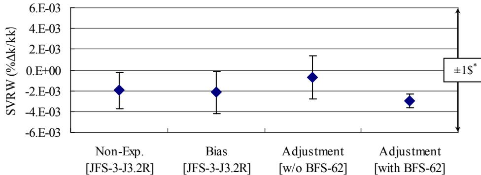
**Fig. 2** Nominal values and the predicted uncertainties for SVRW (Sodium-voided in all fuel region & the axial blanket) [ $\beta_{\text{eff}} = 5.87 \times 10^{-3}$ ]
