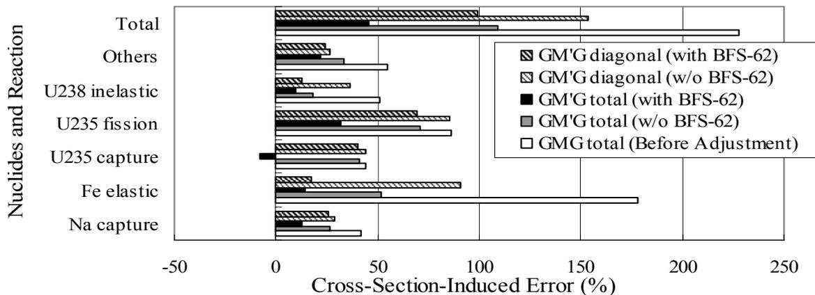
**Fig. 3** Breakdown of the predicted uncertainty into nuclides & reactions (SVRE for all the fuel regions and the upper blanket)
