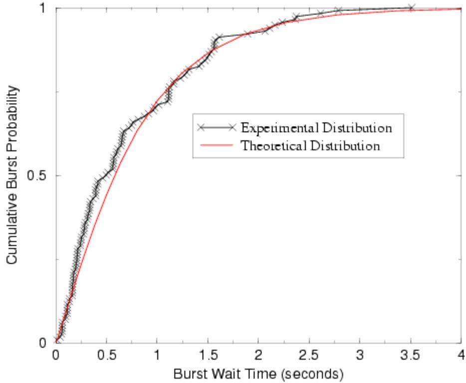
**Fig.2** Experimental and calculated neutron burst cumulative distribution probability versus wait time.
