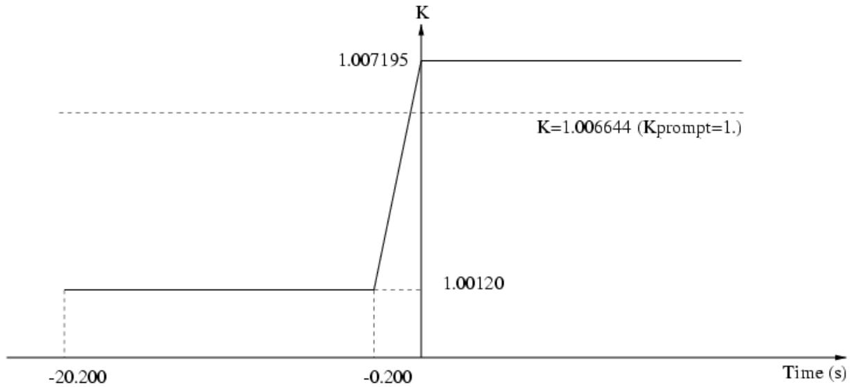
**Fig.1** Time dependent total multiplication coefficient K value used in the numerical application.
