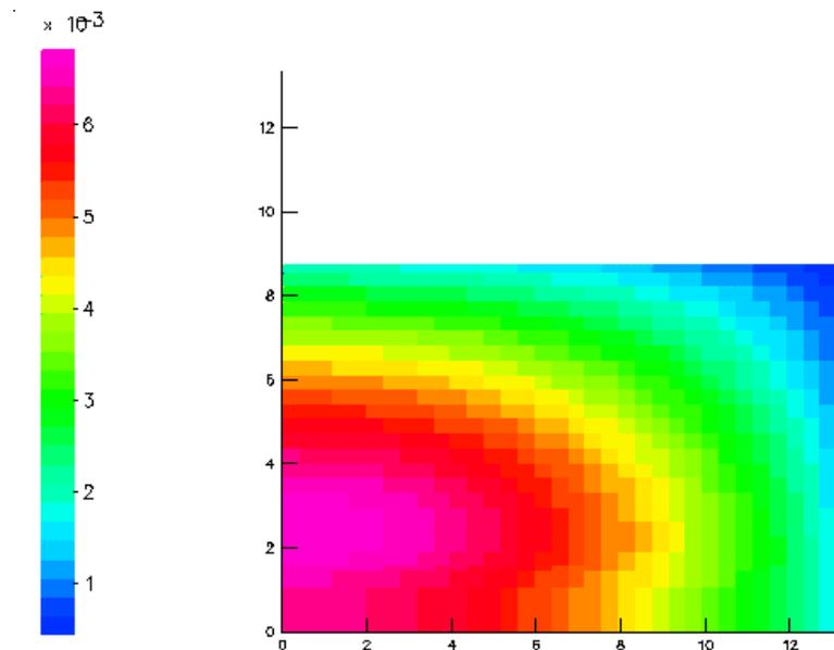
**Fig.4** Caliban initiation probability map for a single initial fission neutron in each cell.
