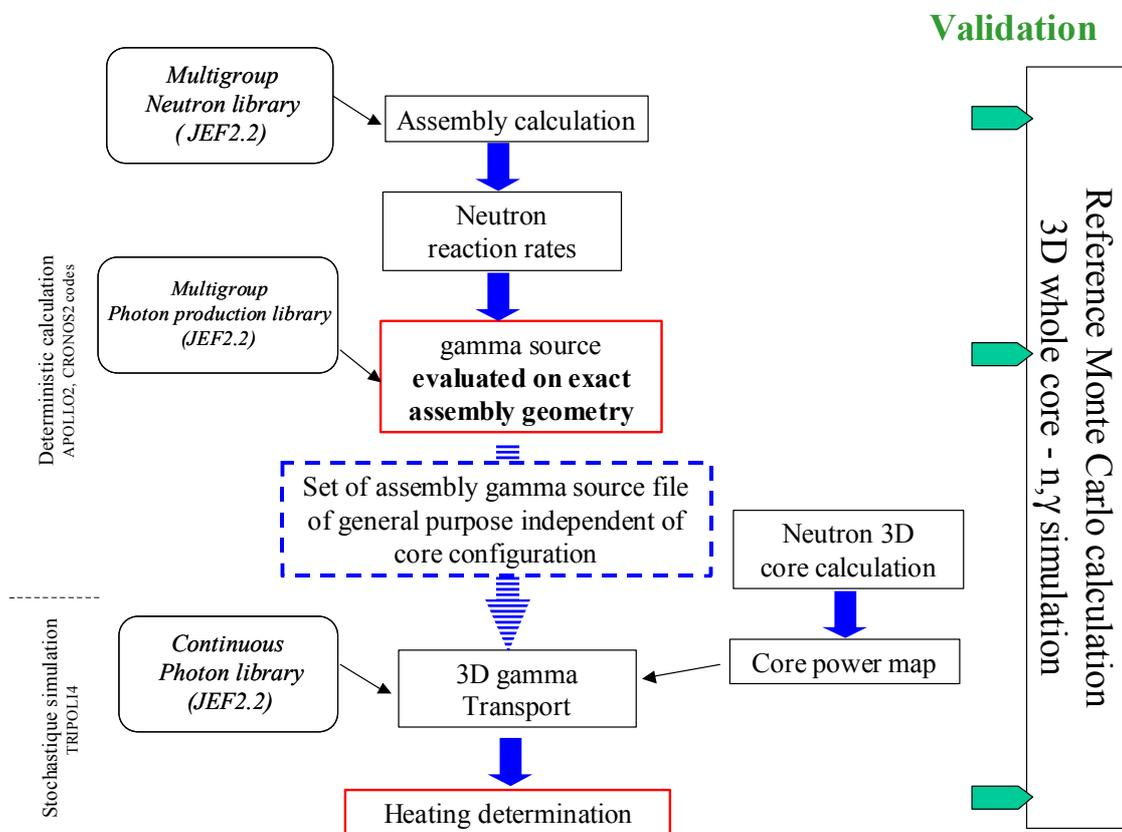
**Figure 4 : The photon calculation scheme**
