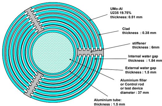
**Figure 1 : Cross-section of the JHR assembly**
