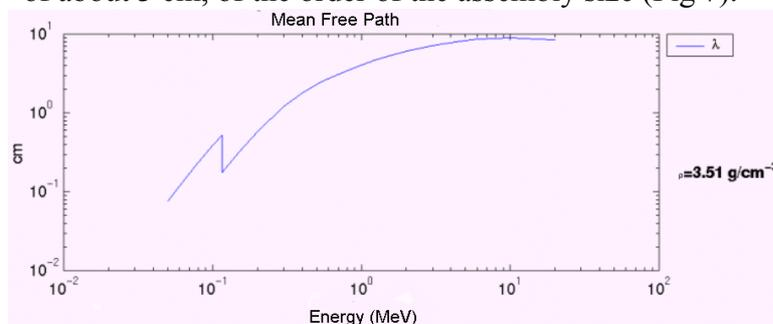
**Figure 6 : Gamma mean free path in standard fuel assembly**
