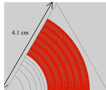
**Figure 7 : Example of  $\gamma$ -source homogenization in assembly fuel area (red)**
