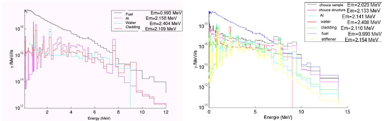
**Figure 5 : Example of gamma source spectra in fuel (left) and single CHOUCA (right) assembly with average energy**
