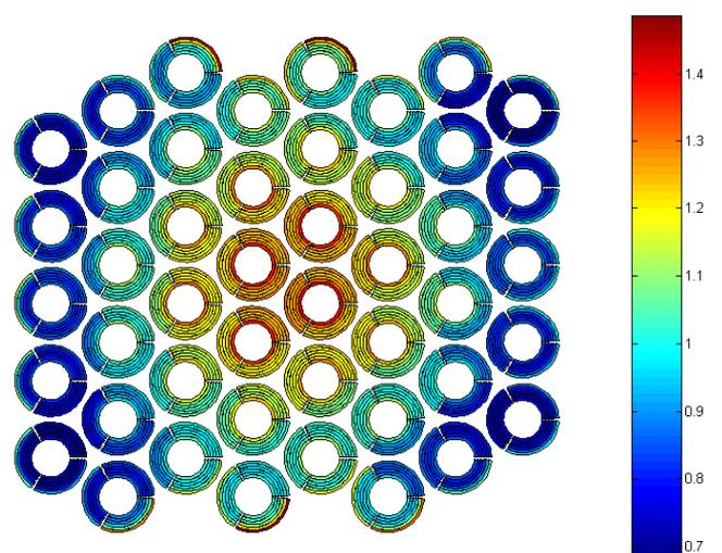
Figure 9 : Fine power distribution per plate
