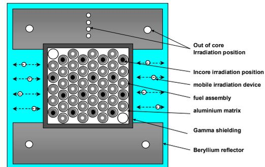
**Figure 2 : Cross-section of the JHR core**
