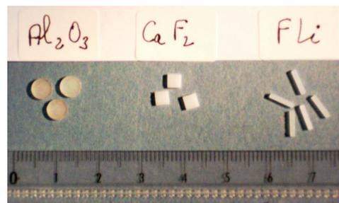
**Figure 12 : close vue of a set of different TLD**
