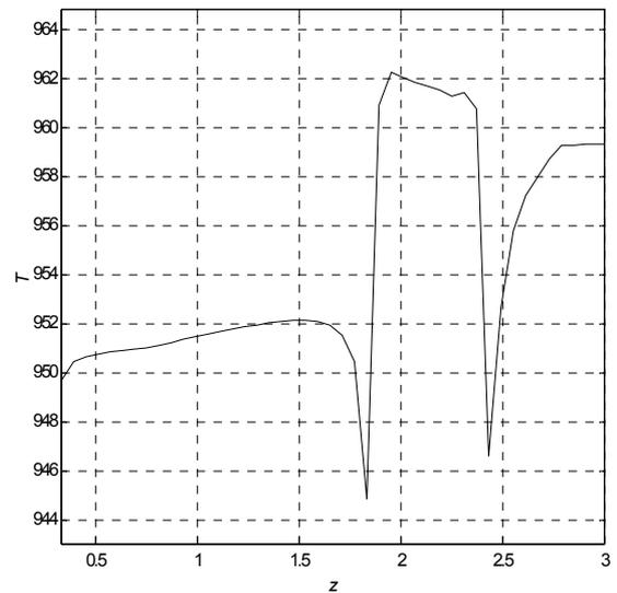
Fig.4. Temperature of outer surface of the wall separating the Outer and Inner Cores, K
