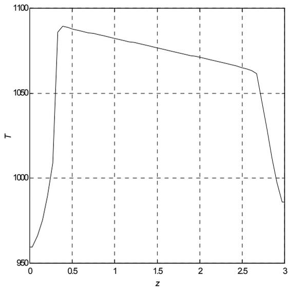
Fig.3. Temperature of Outer Core sidewall, K
