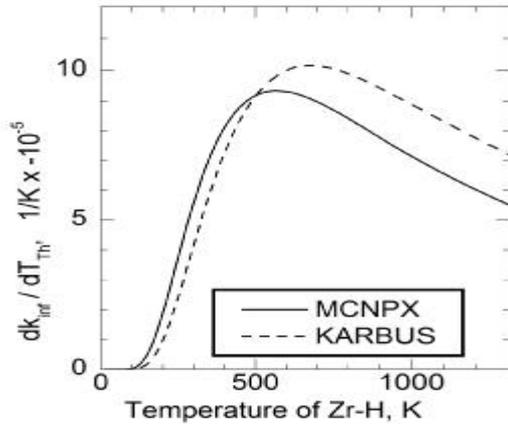
**Fig 5:** Thermal up-scattering fitting curve of MCNPX and KARBUS-TWODANT data points for 2D Model. The governing fitting formula is based on GA (U235 & U238 at 300 K)
