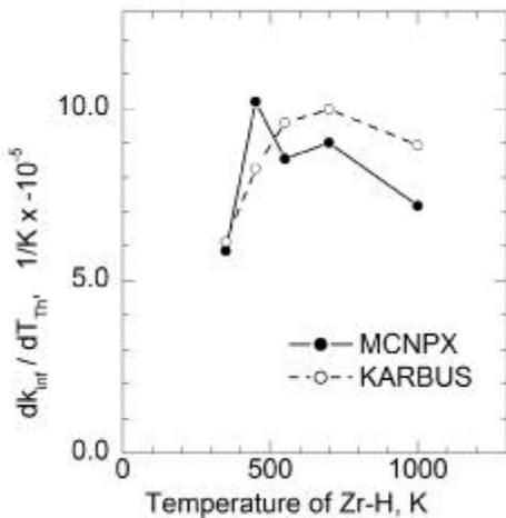
**Fig 7:** Comparison of the thermal up-scattering between MCNPX and KARBUS-TWODANT for 2D Model (U235 & U238 at 300 K)
