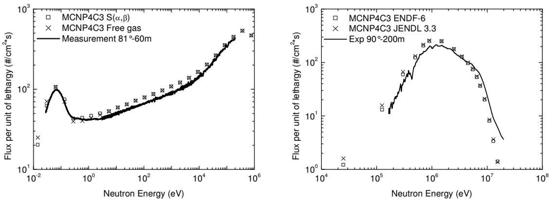
**Fig.2** Neutron flux per unit of lethargy in the flight-path a)  $81^\circ$ - 60 m of the moderated neutron spectrum b)  $90^\circ$ - 200 m of the fast neutron spectrum
