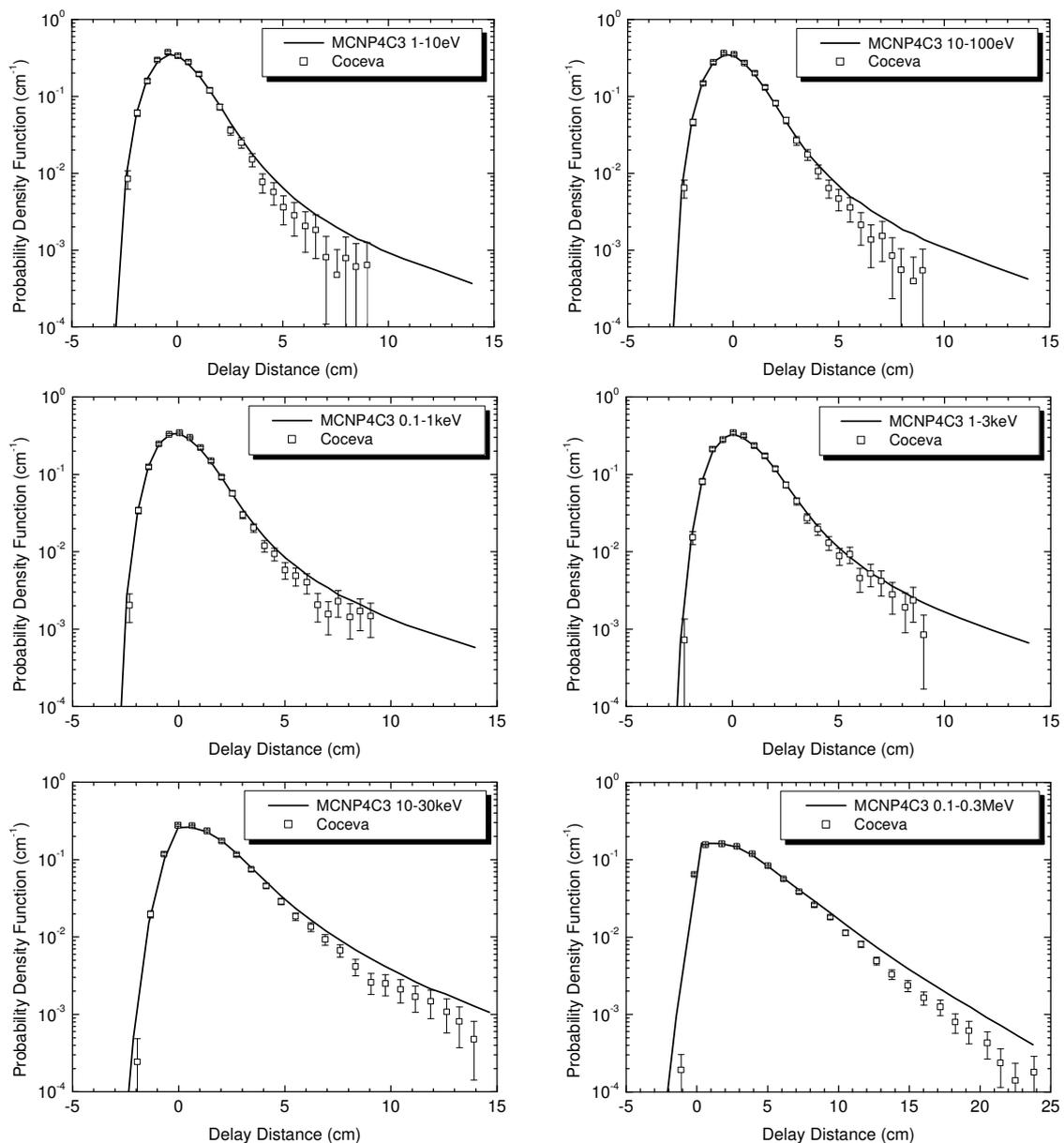
**Fig.3** Resolution functions for the moderated neutron spectrum at 81°
