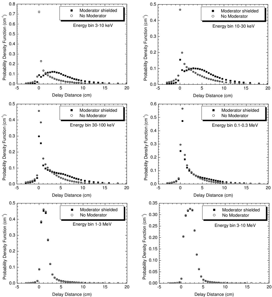
**Fig.4** Resolution functions for the direct neutron spectrum at  $90^\circ$
