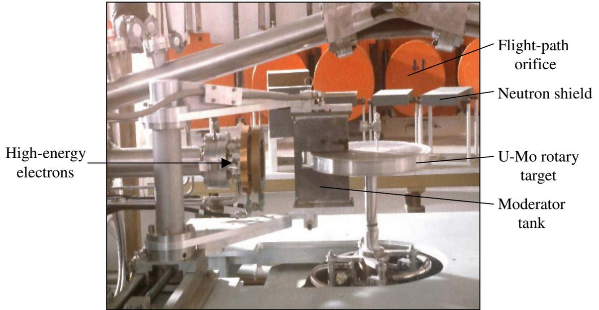
**Fig.1** The GELINA neutron rotary target
