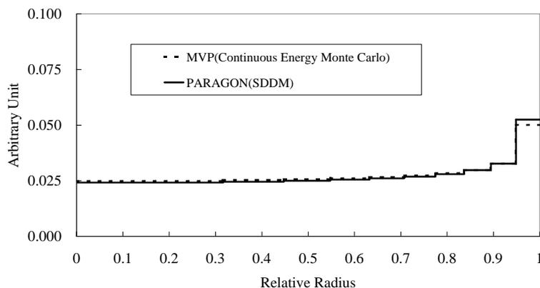
Fig. 2 U-238 Absorption Rate Distribution at Cold Zero Power (Pellet/Cladding/Moderator=300k/300k/300k)
