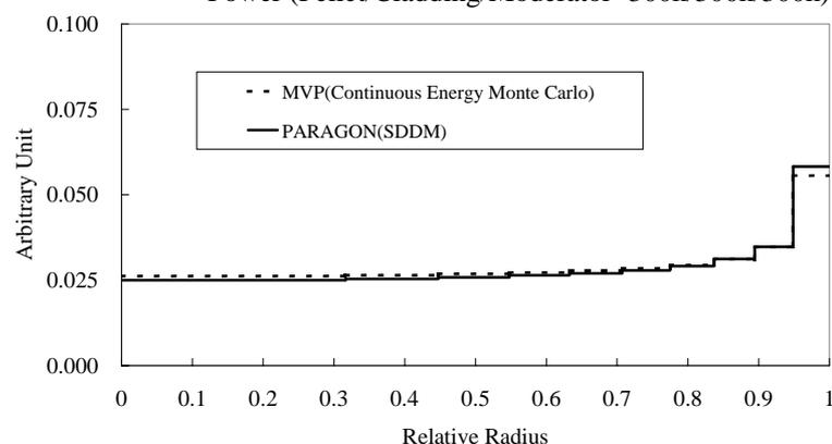
Fig. 3 U-238 Absorption Rate Distribution at Full Power (Temperature profile came from a fuel performance code)
