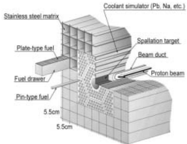
**Fig.6** Pin-type fuel partial loading section for TEF-P
