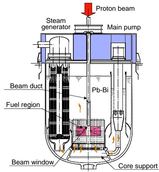
**Fig.2** Conceptual design of ADS
