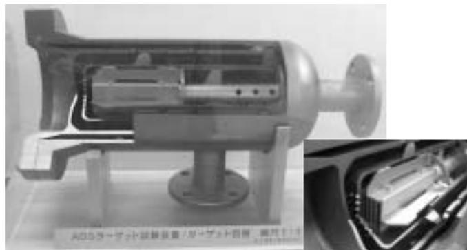
**Fig.7** Pb-Bi spallation target model (1/1 scale)
