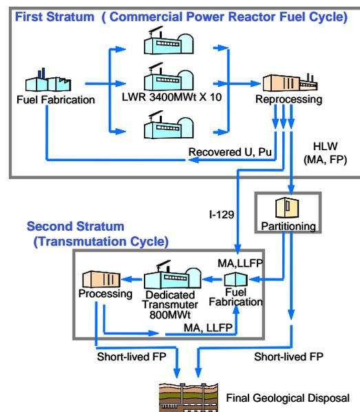
**Fig.1** Double-Strata Fuel Cycle Concept
