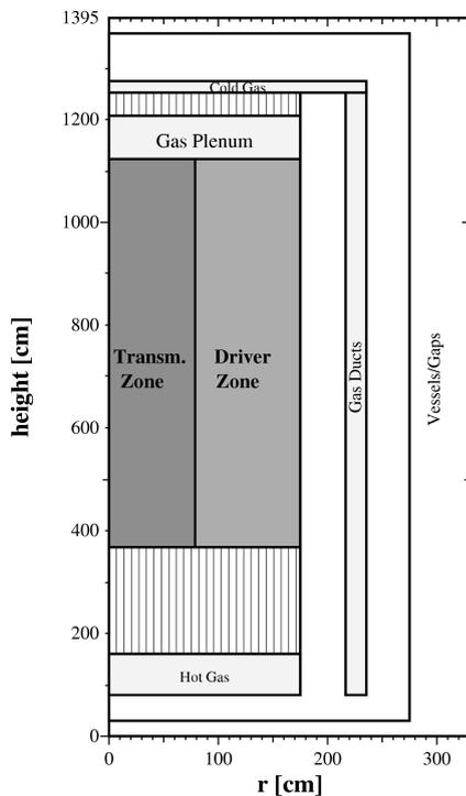
Fig. 1 Calculational model of the 268 MWth PBMR design
