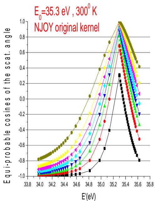
**Fig. 2:** Differential scattering cosine bins based on the original NJOY kernel at 300<sup>0</sup> K
