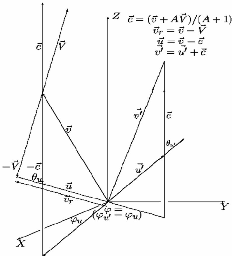
**Fig. 1:** Definition of Velocities and angles after and before the neutron scattering.
