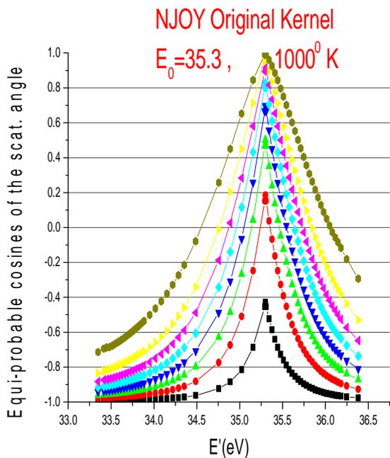
**Fig. 4:** Differential scattering cosine bins based on the original NJOY kernel at 1000<sup>0</sup> K
