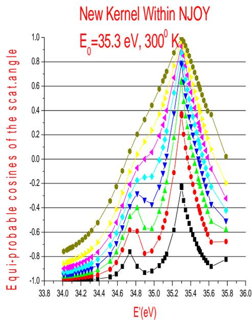
**Fig. 3:** Differential scattering cosine bins based on the new inserted formula in NJOY at 300<sup>0</sup> K
