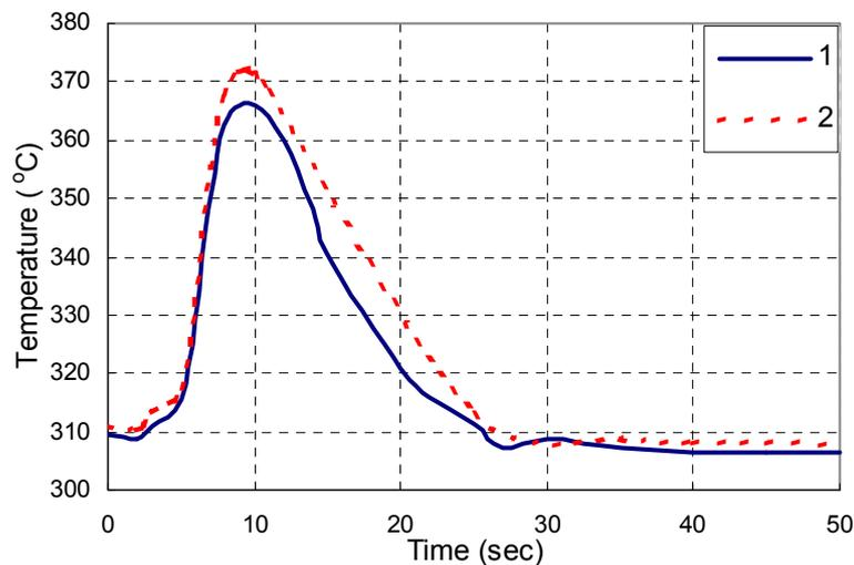
**Fig.12** Peak cladding temperature in fuel rod. Number of rod: 1 – 12; 2 – 6 (see Figure 9).
