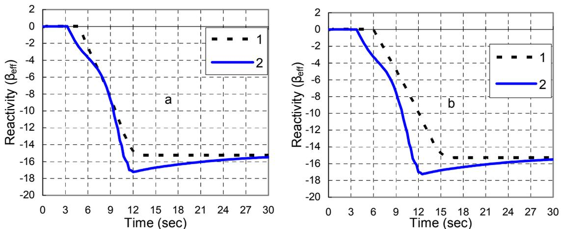
**Fig.4** Total reactivity behavior during MCR bank withdrawal:
