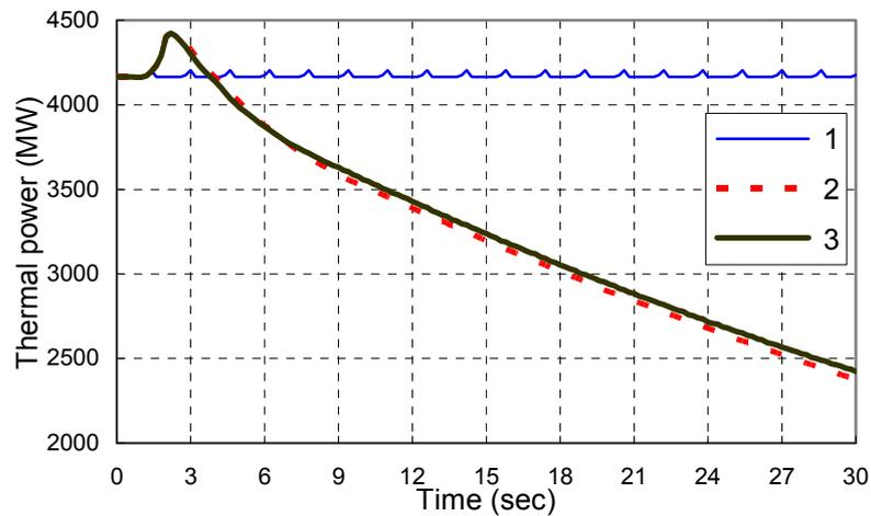
**Fig.7** Total reactor power behavior during shortened absorber rod dropout:
