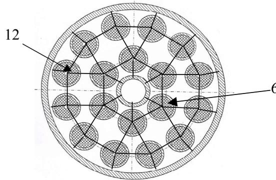
**Fig.9** Cross section of the RBMK-1500 fuel channel model with VIPRE-02.
