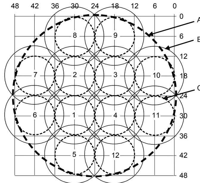
**Fig.1** RBMK-1500 core and CPS zones in INPP coordinates:
