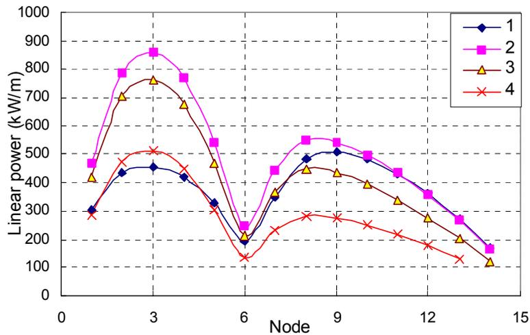
**Fig.11** Linear power in fuel channel 41-32. Transient time: 1 – 0 sec, 2 – 1.6 sec, 3 – 7 sec, 4 – 40 sec.
