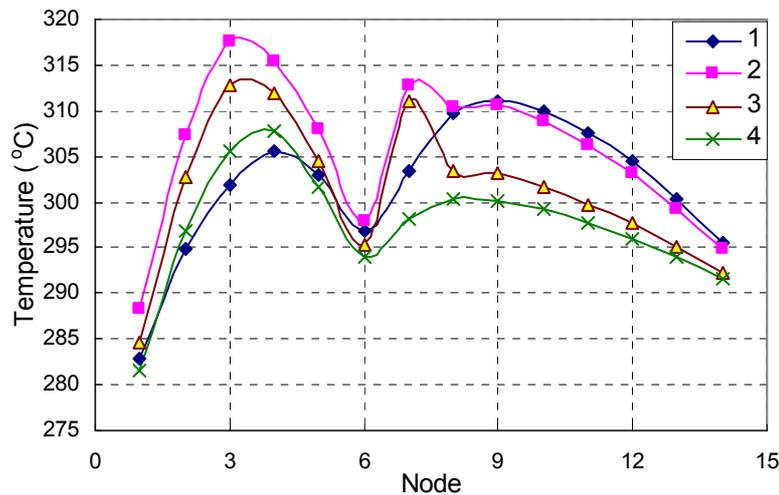
**Fig.13** Axial cladding temperature profile for the fuel rod No.6. Transient time:
