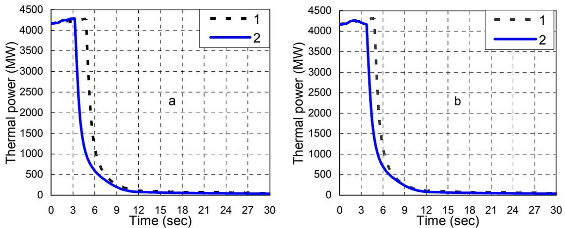
**Fig.3** Total reactor power behavior during MCR bank withdrawal:
