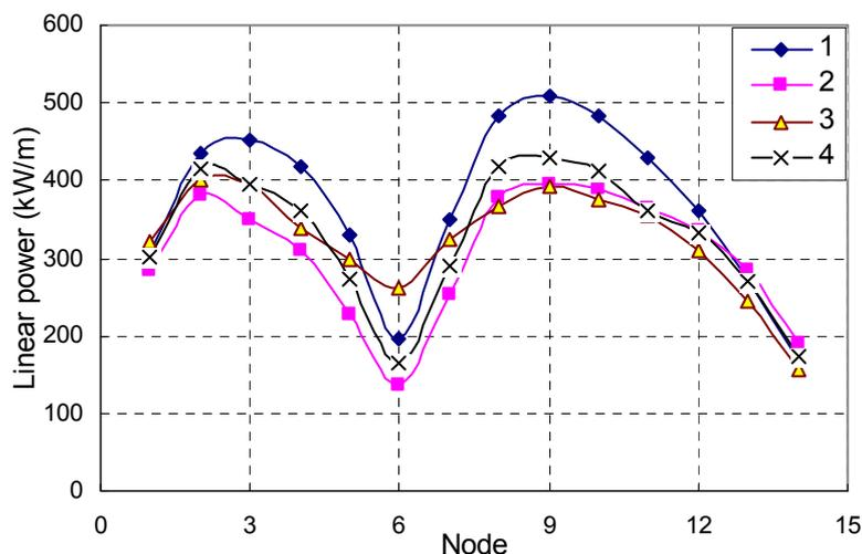
**Fig.10** Initial axial power profiles at fuel assemblies related in INPP coordinates:
