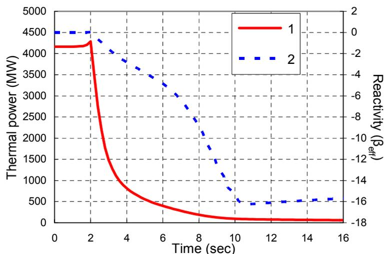
**Fig.6** Simulation of drop out of the single short control rod:
