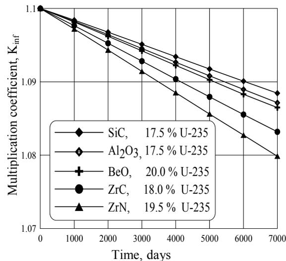
**Fig.2** Dependence of multiplication factor versus irradiation time for different matrix materials
