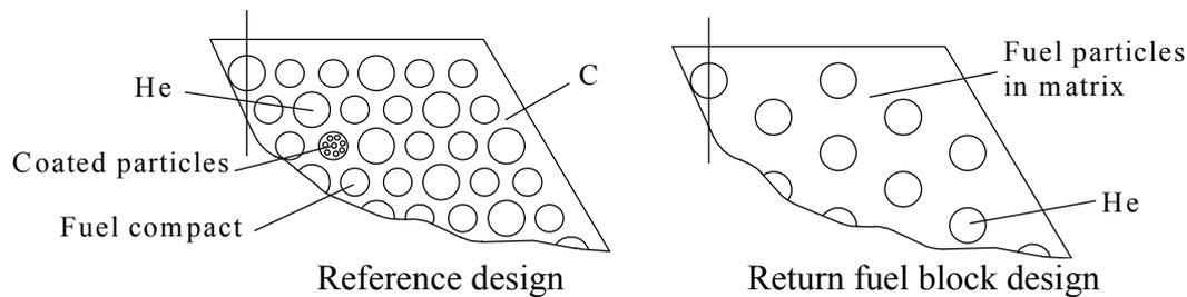
**Fig.1** Reference and return configurations of fuel block
