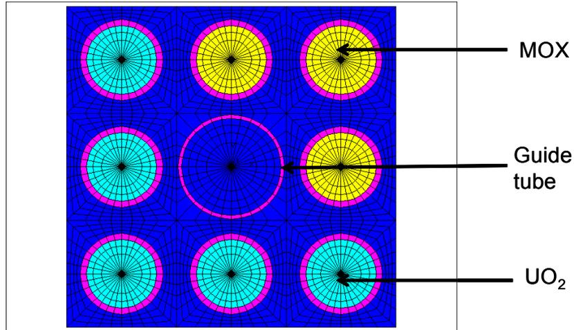
**Fig.2** UO<sub>2</sub>/MOX 3x3 Geometry
