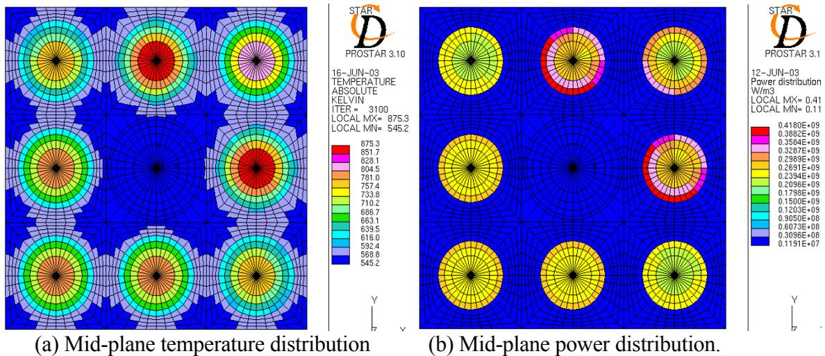
**Fig.3** Results for UO<sub>2</sub>/MOX assembly.
