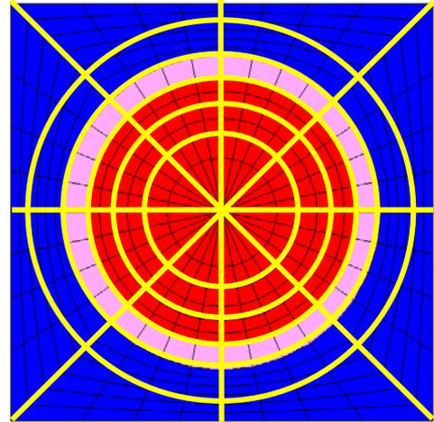
**Fig.1** The CFD Mesh (black lines), The Zone Set Boundaries for Coupled Calculations (yellow lines).
