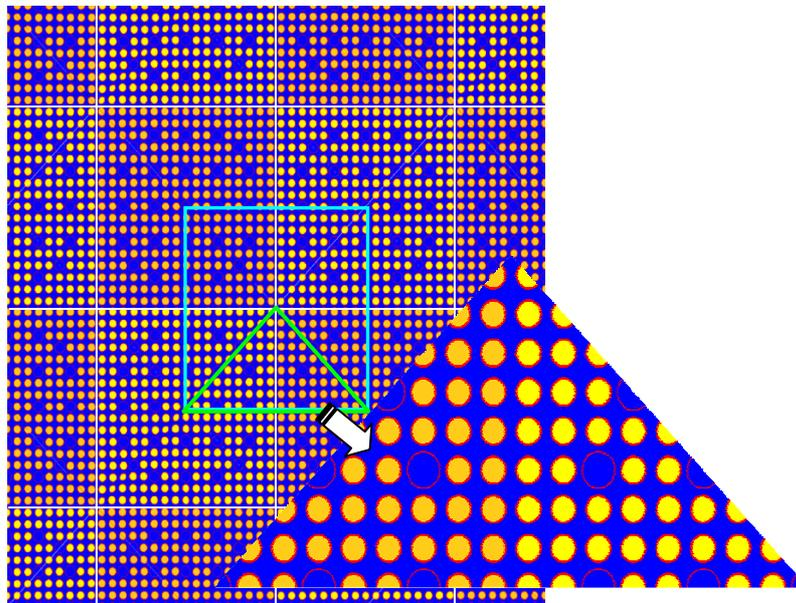
**Fig.4** The checkerboard core configuration. The blue square represents the symmetric segment used in the DeCART model; the enlarged green triangle shows the symmetric segment for CFD simulations. The orange color indicates  $\text{UO}_2$  fuel pins, the yellow color indicates MOX fuel pins.
