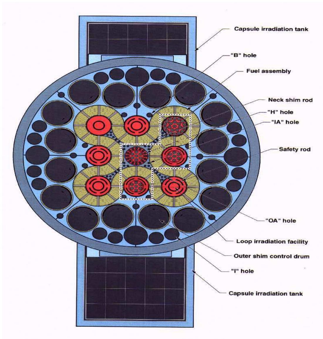
**Fig.1** Horizontal Cross-Section View of ATR Core
