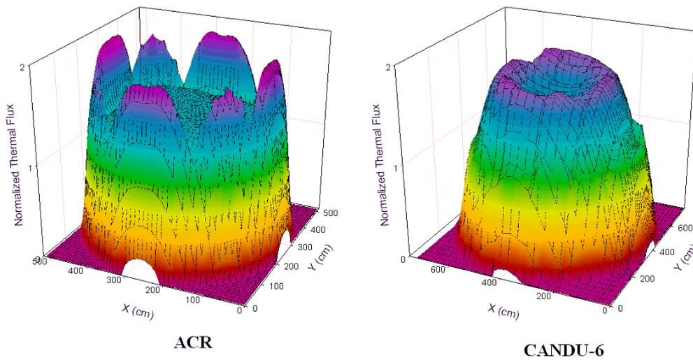
Fig. 5 Radial Thermal Flux Profiles in ACR-700 and CANDU-6
