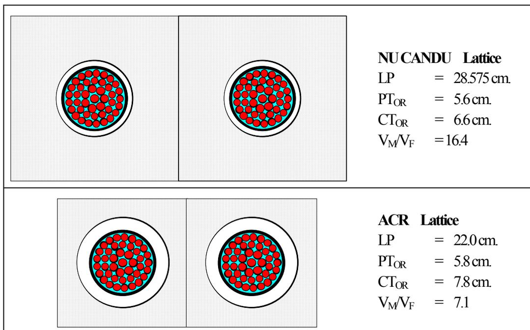
**Fig. 3** ACR and NU CANDU Lattice-Cell Configurations
