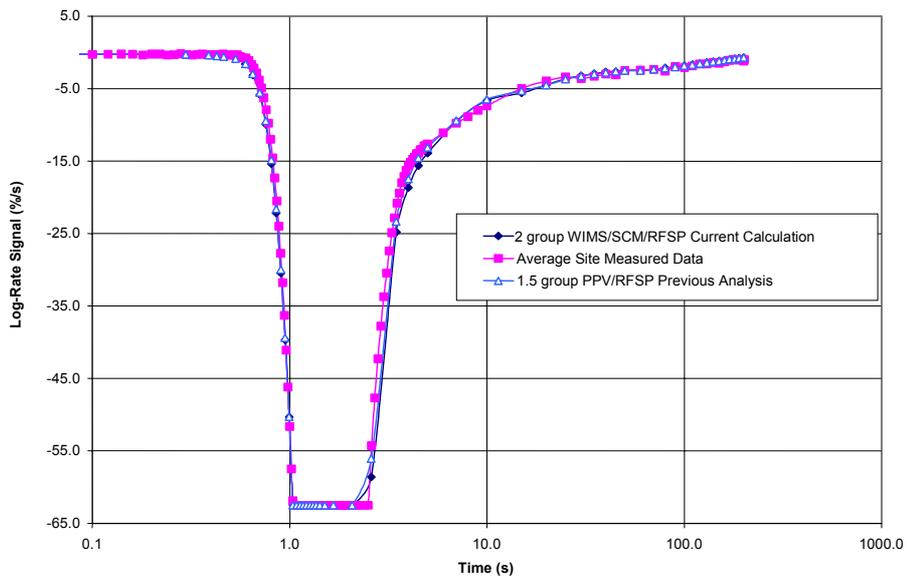
**Fig. 1 Comparison Between Measured and Calculated “Log-Rate Signal: Ion Chamber H”**
