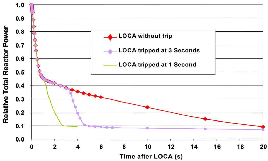
Fig.4 Reactor Power Transient in ACR-700 After Full-Core LOCA
