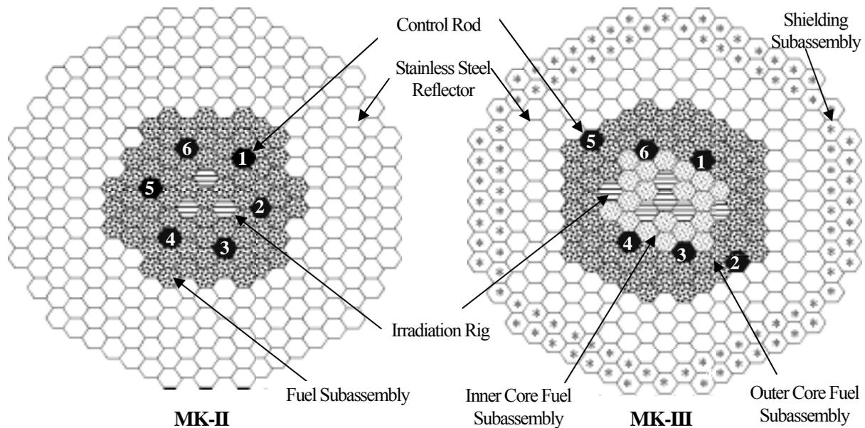
**Fig.1** Comparison of JOYO MK-II and MK-III cores used in the core design
