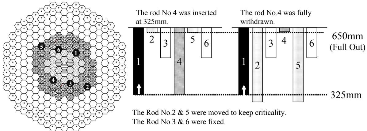
**Fig. 3** Control rod pattern of shadowing effect measurement
