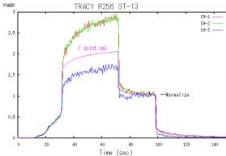
Fig.5 Analysis result for Case (2) by one-point kinetics method
