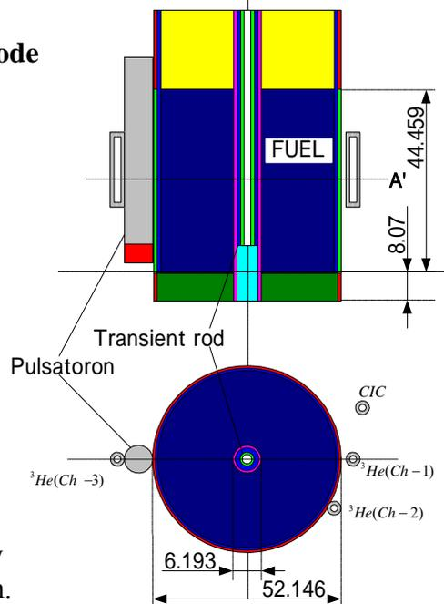
Fig.6 MVP calculation geometry
