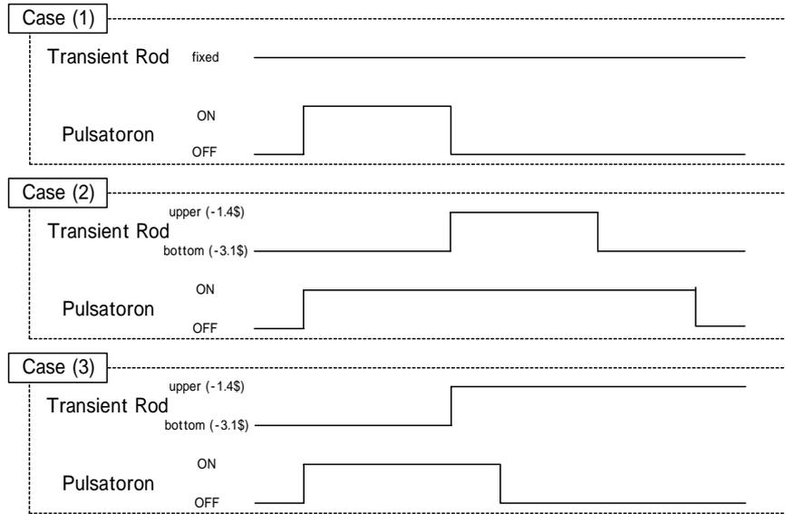
Fig.3 Experimental patterns simulating ADS operation
