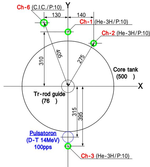
Fig.2 Experimental arrangement using TRACY and Pulsatoron
