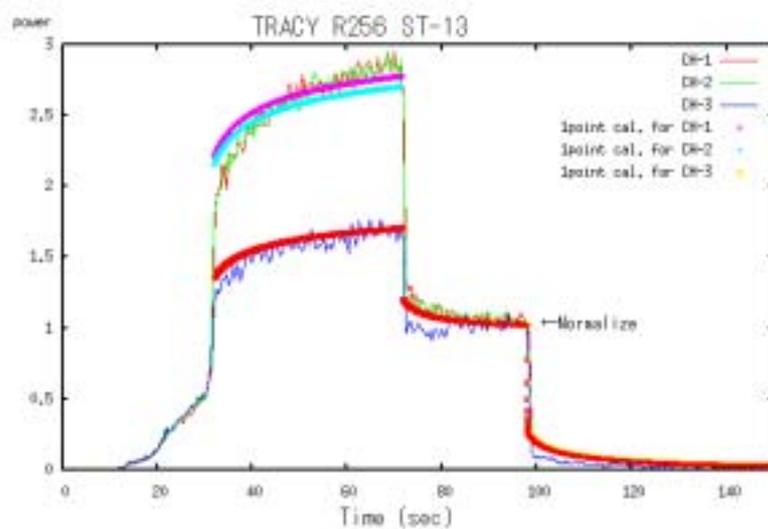
Fig.8 Calculated time response of He-3 detectors by the modified method using MVP
