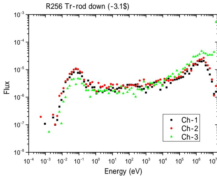
Fig.7 Calculated energy spectrum at He-3 detectors by the modified method using MVP
