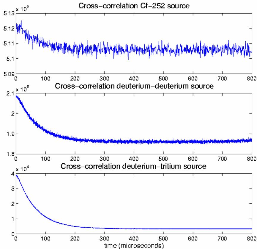
**Fig 2** Cross Correlation of a source driven system with 3 different sources
