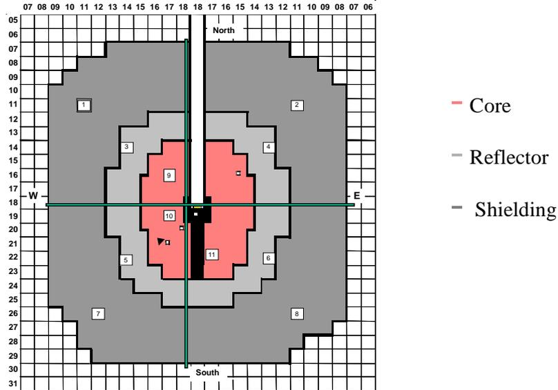
**Fig. 1:** Horizontal cross section at mid-plane of the MASURCA core with the detector positions indicated.
