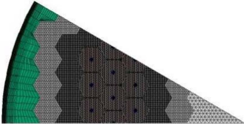
Figure 3: View of the region partition for the 1/12 symmetry HTGR. The central fuel region intersects 10 fuel assemblies.
