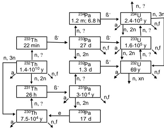
**Fig. 1** Schematic view of the thorium fuel cycle. Production and decay modes, as well as half-lives are shown for each isotope. The  $^{233}\text{Pa}$  isotope is highlighted.
