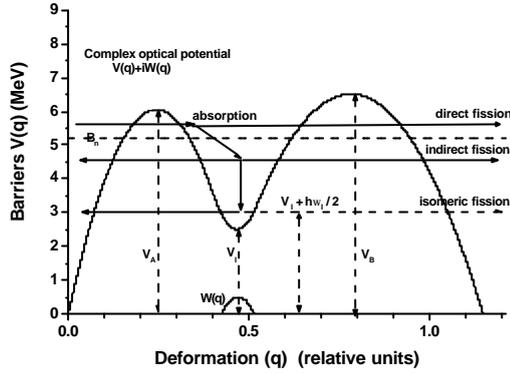
**Fig. 7** Schematic view of the double humped fission barrier with all the possible decay mechanism involved.
