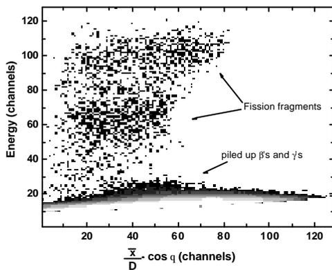
**Fig. 5** Plot of the pulse height distribution versus the particle range. This two-dimensional distribution was used to identify the fission fragments.
