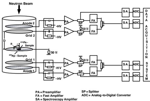
**Fig. 3** Schematic view of the experimental set-up.
