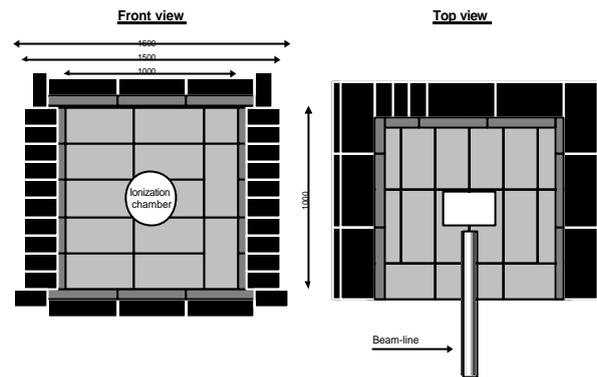
**Fig. 4** Schematic view of the radiation shielding.
