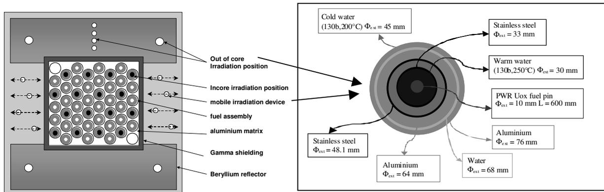
Figure 2 : Cross section of an experimental device “griffon” outside the JHR core
