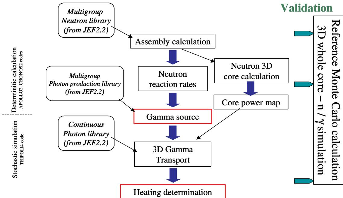
Figure 6 : Nuclear heating scheme
