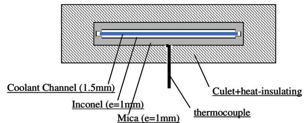
Figure 9 : Test section geometry
