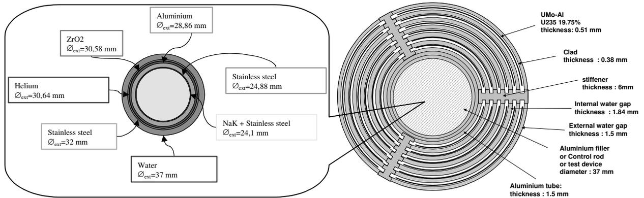
Figure 1 : Cross section of an experimental device “single chouca” inside the JHR assembly
