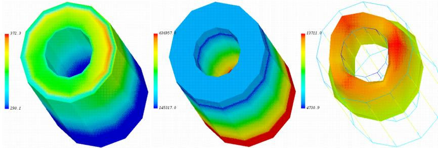
Figure 10 : FLICA4 hot element results (from left to right, temperatures, pressure, mass flow rate)
