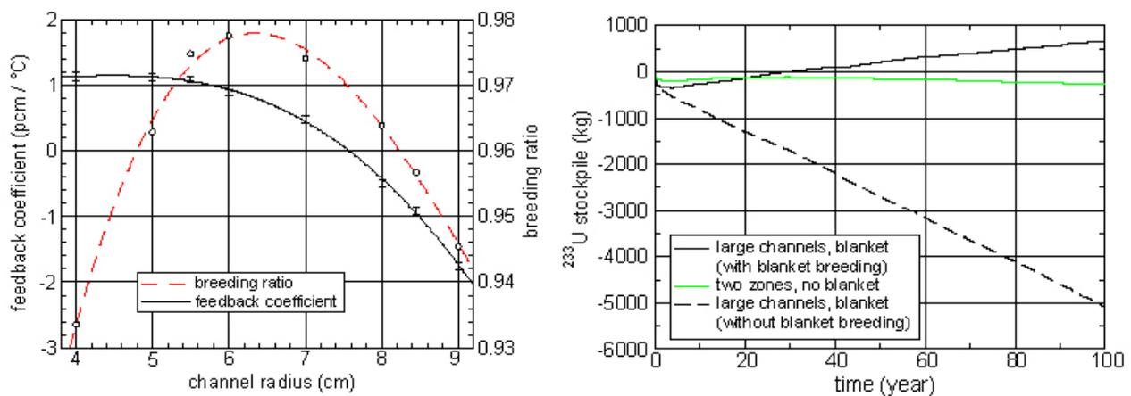
**Fig. 5** (left) Impact of the channel radius on the temperature coefficient and the breeding ratio (for a 6 months reprocessing, Pa and TRUs extracted, no blanket) (right) Fissile materials stockpile for different core configurations (with and without Thorium blanket)
