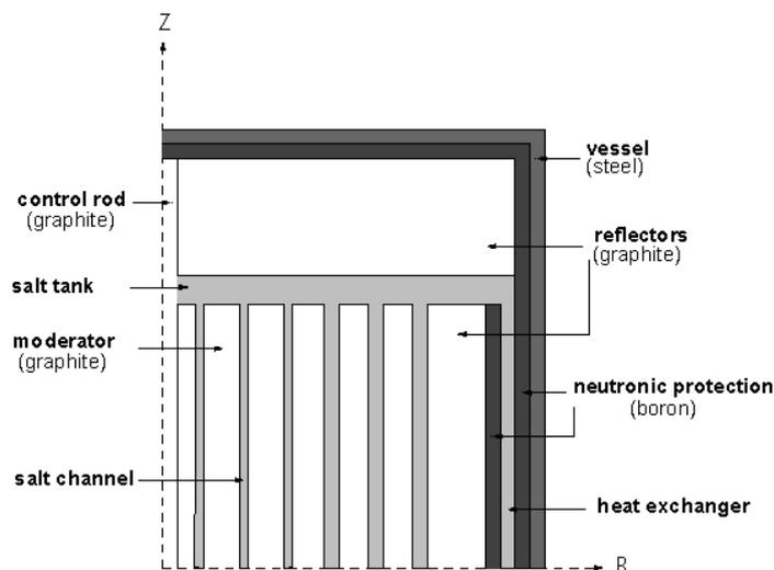
**Fig. 1** MSBR vertical slice of the core
