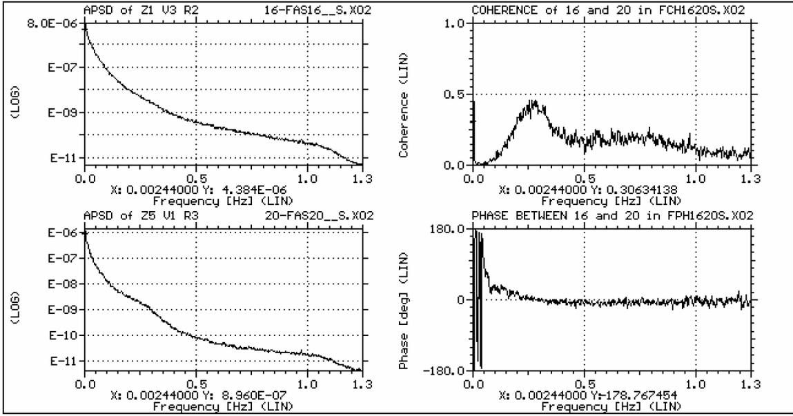
**Fig. 7** Normalized APSDs, coherence and phase functions of ICFD noise signals from zones #1 and #5 in the Darlington Unit 3 CANDU reactor
