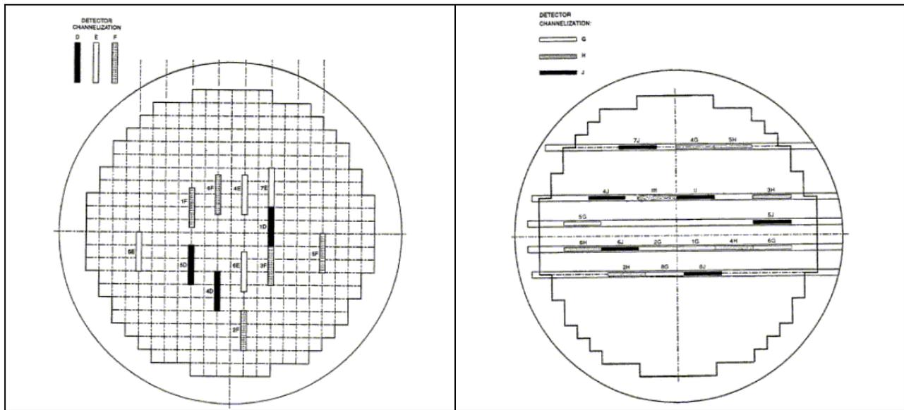
**Fig. 3** Overview of the position of the ICFDs used by the SDSs (Vertical Flux Detectors – or VFDs – for SDS-1 on the left hand-side, and Horizontal Flux Detectors – or HFDs – for SDS-2 on the right hand-side). [2]
