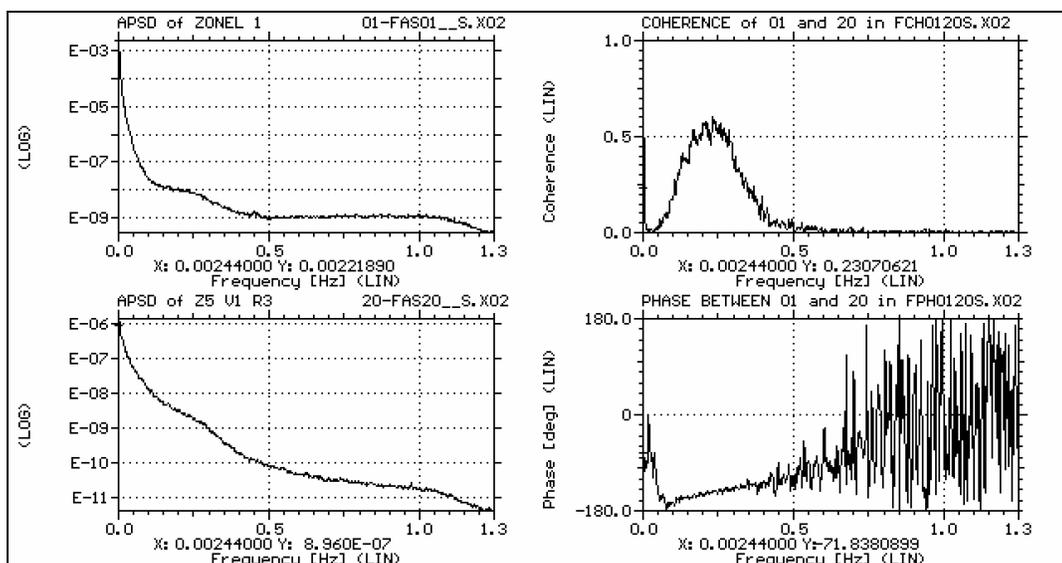
**Fig. 6** Normalized APSDs, coherence and phase functions of the liquid zone level noise from zone #1 and ICFD noise from zone #5 in the Darlington Unit 3 CANDU reactor
