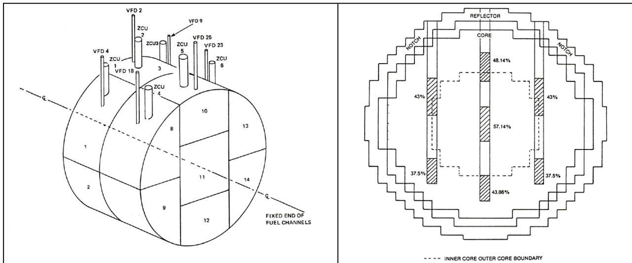
**Fig. 1** Overview of the position of the tubes (abbreviated as ZCU – Zone Control Units) containing the light water compartments (on the left hand-side), and overview of the position of the water compartments in each tube (on the right hand-side). [2]
