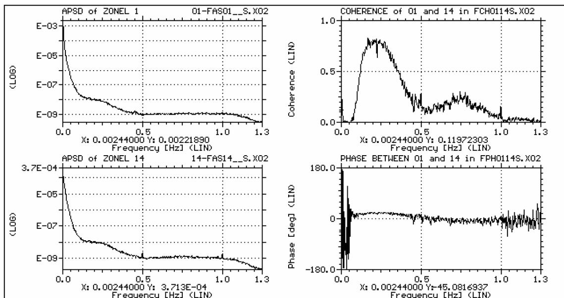
**Fig. 2** Normalized APSDs, coherence and phase functions of noise signals of liquid zone levels from zones #1 and #14 measured in the Darlington Unit 3 CANDU reactor
