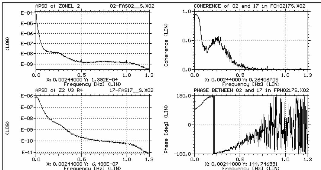
**Fig. 5** Normalized APSDs, coherence and phase functions of the liquid zone level noise and ICFD noise measured in zone #2 in the Darlington Unit 3 CANDU reactor
