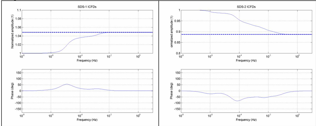
**Fig. 4** Calculated Bode diagrams of the normalized nominal dynamic transfer function of the ICFDs used in SDS-1 (on the left hand-side), and in SDS-2 (on the right hand-side). The dashed lines represent the relative prompt fraction of the detectors.
