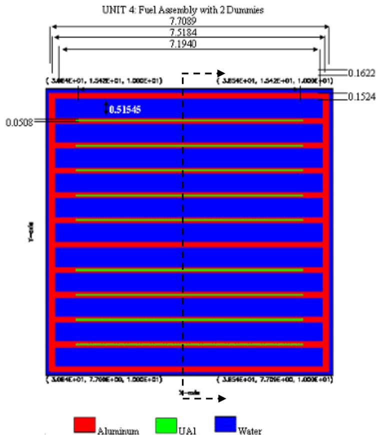
**Fig 4** Two dimensional cross section of the PUR-1 unit 4
