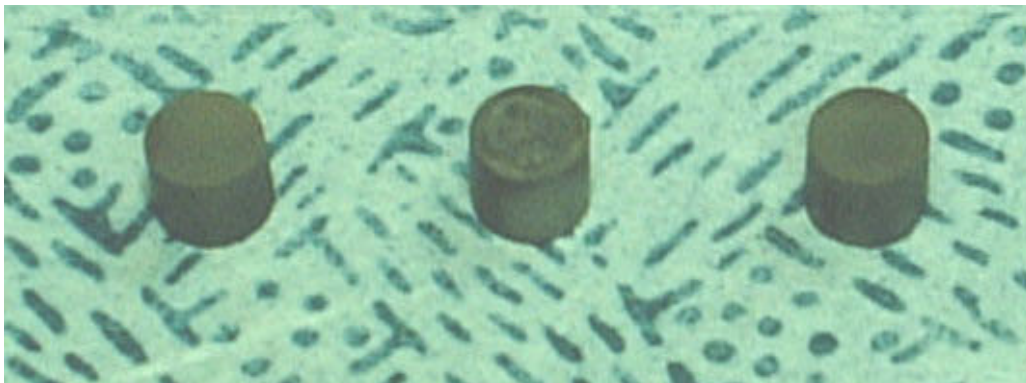
Figure 17: Initial fuel pellets of UO_2 and (UO_2 + 4\% ThO_2)
