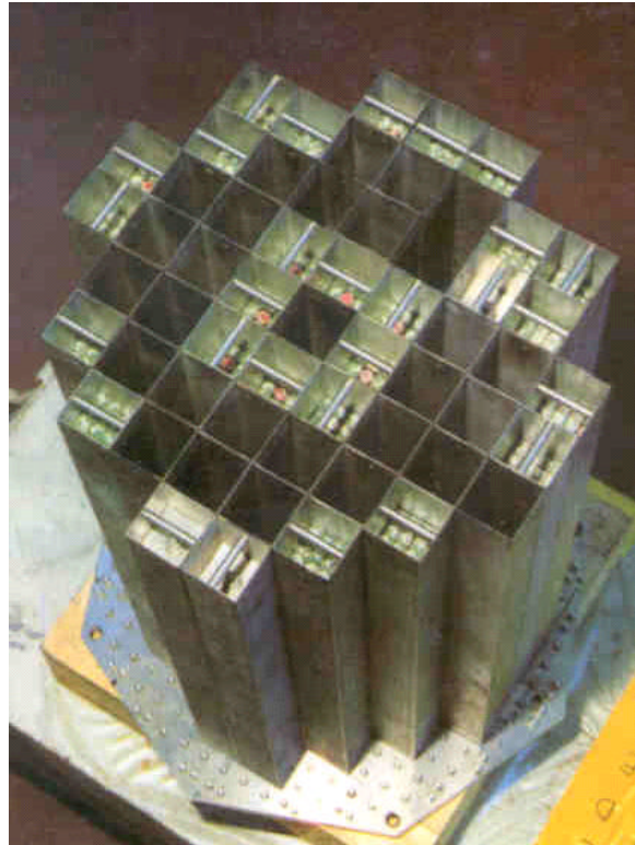
Figure 8: Fast spectrum lattice in MINERVE (ERMINE)
