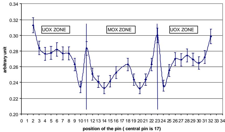
**Figure 9:** Horizontal radial power distribution in R1-MOX configuration
