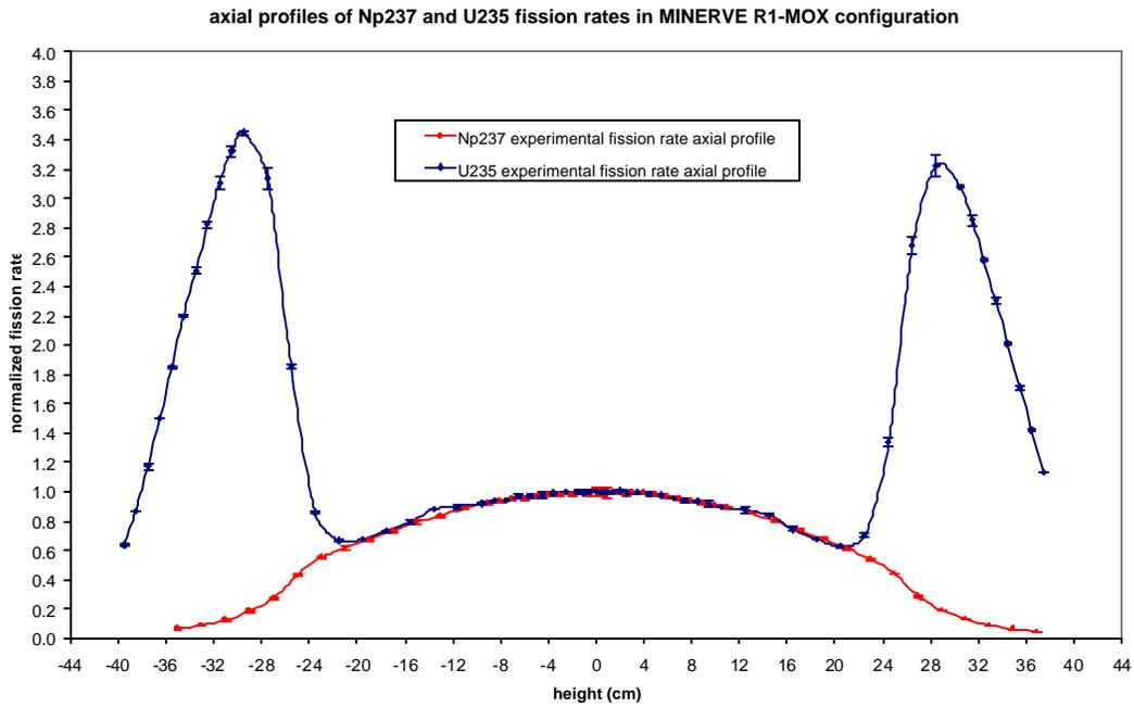
**Figure 5:** axial distribution of  $^{237}\text{Np}$  and  $^{235}\text{U}$  fission rate
