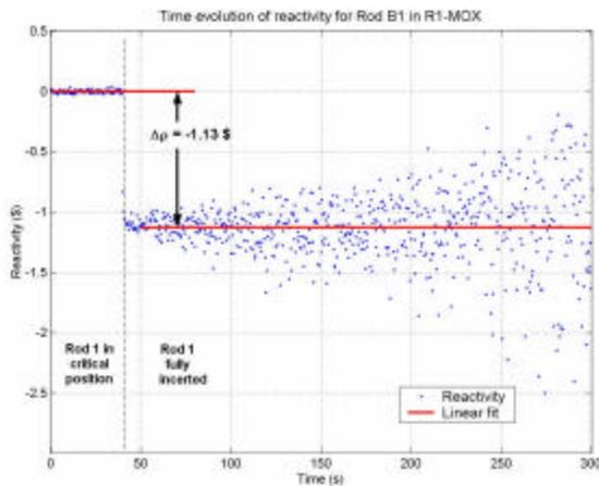
**Figure 3:** Example of reactivity worth determination using the rod drop technique
