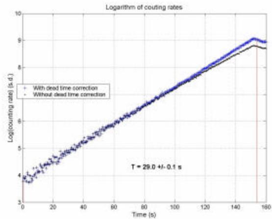
**Figure 4:** Example of stable reactor period adjustment
