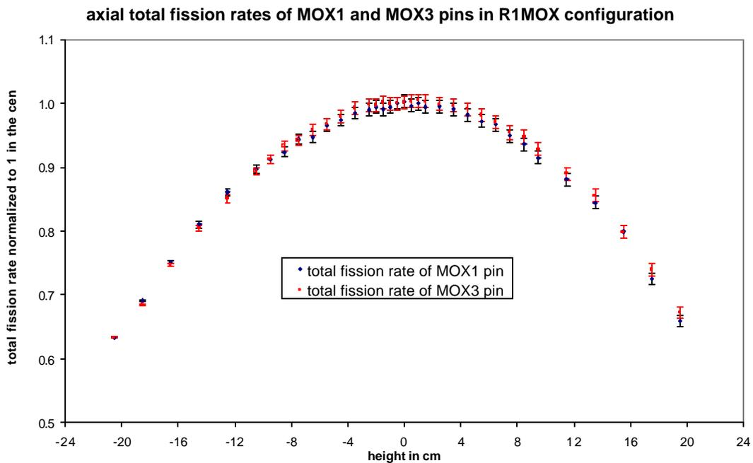
**Figure 6:** axial total fission rate of *MOX1* and *MOX3* pins
