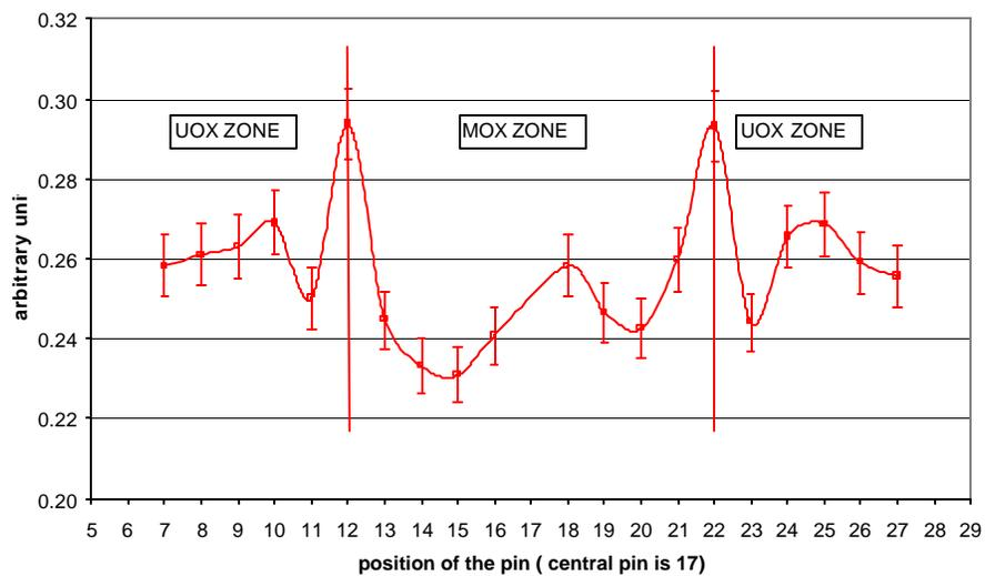
**Figure 10:** Diagonal radial power distribution in R1-MOX configuration
