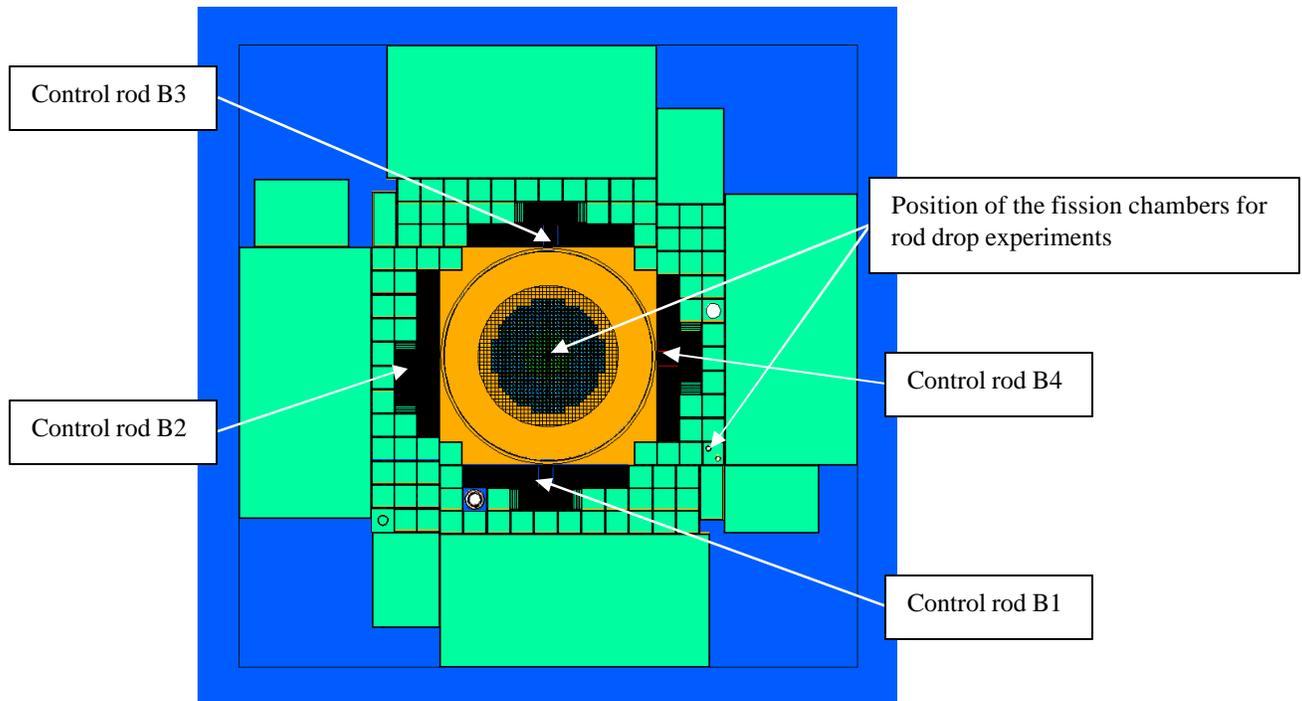
**Figure 1:** MCNP Model of MINERVE Reactor with R1-MOX Loading (radial view)
