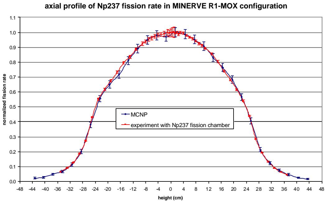
Figure 11: comparison of calculated and measured axial profile of Np-237 fission rate in R1-MOX
