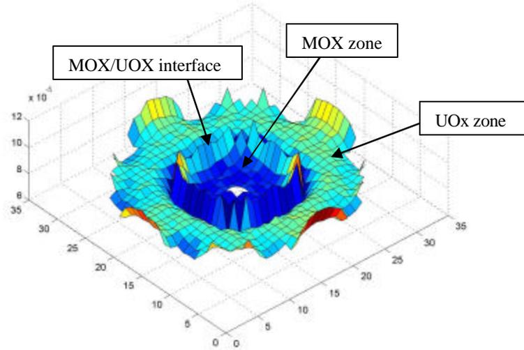
**Figure 17:** power profile in R1-MOX configuration, obtained by MCNP calculation
