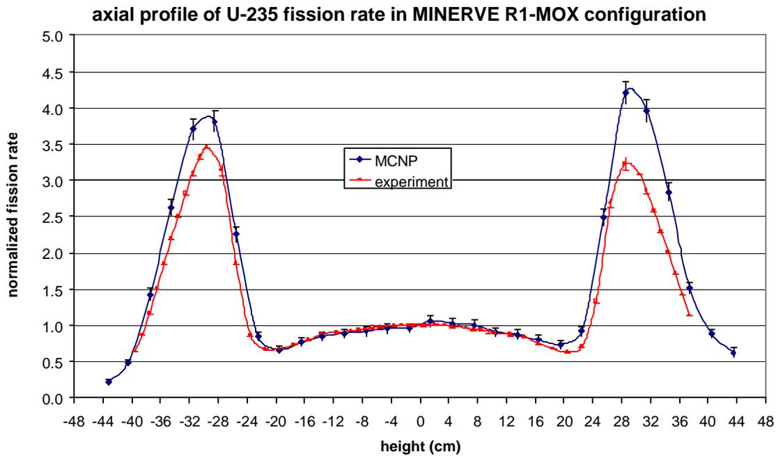
Figure 12: comparison of calculated and measured axial profile of U-235 fission rate in R1-MOX
