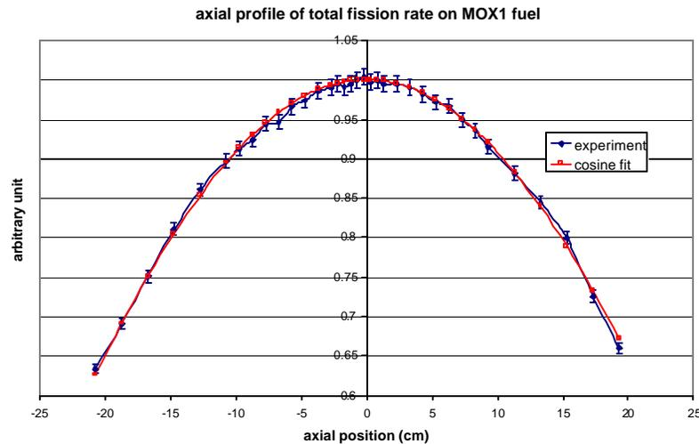
**Figure 7:** axial profile of MOX1 pin and cosine fit
