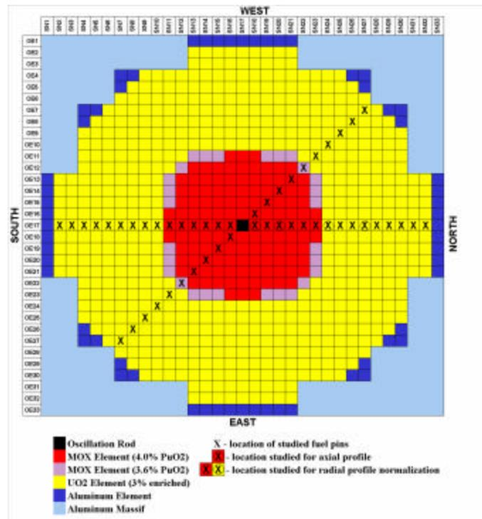
**Figure 2:** Locations of the Studied Fuel Pins for axial profile measurement
