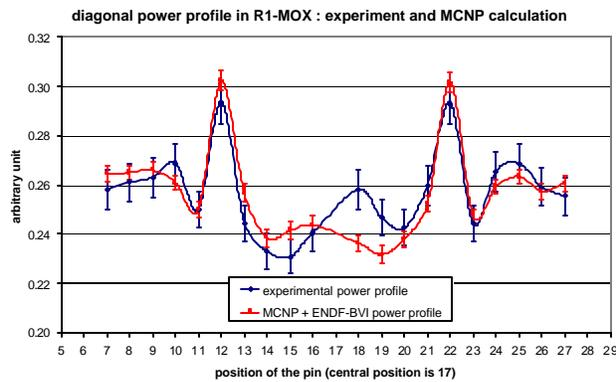
**Figure 15:** Comparison of calculated to experimental diagonal power profile in R1MOX
