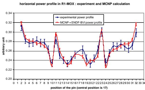
**Figure 13:** Comparison of calculated to experimental horizontal power profile in R1MOX
