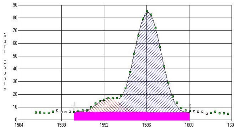
**Figure 8:**  $^{140}\text{La}$  at 1596.17 keV and 2<sup>nd</sup> escape  $^{208}\text{Tl}$  peak for MOX1 fuel pin – counts vs. energy
