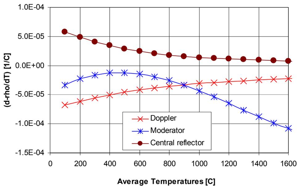
**Fig 7.** Isothermal reactivity temperature coefficients.
