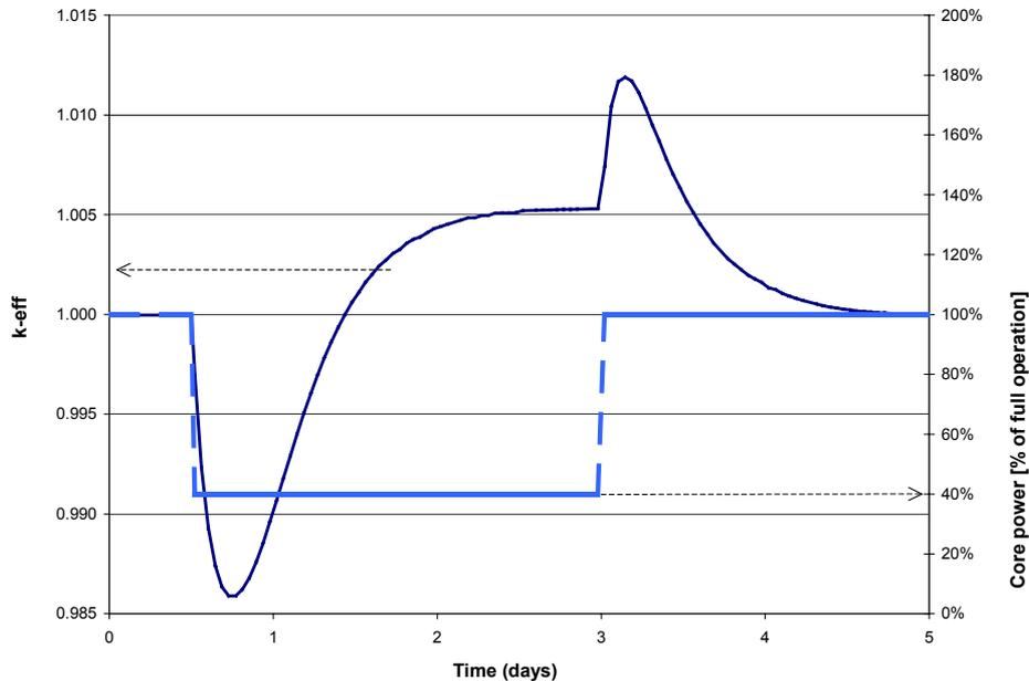
**Fig 6.** Reactivity behaviour due to xenon during a 100%-40%-100% power change
