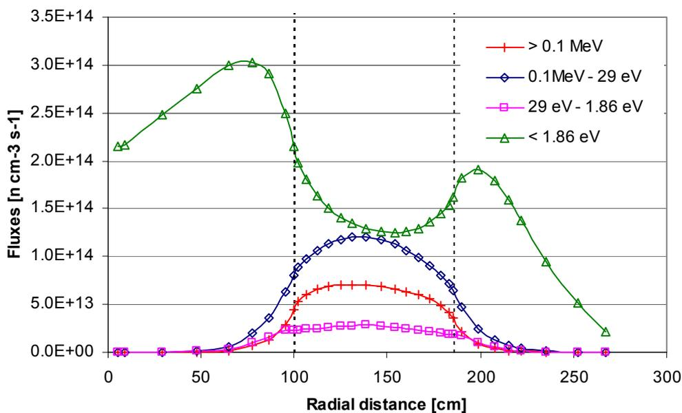
**Fig. 4** Thermal and fast flux distribution in the 400 MWt design
