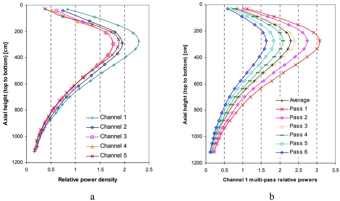
**Fig. 2** (a) Volume averaged relative axial power profile in the radial flow channels, and (b) detailed power distribution of multi-pass fuel batches for channel 1.
