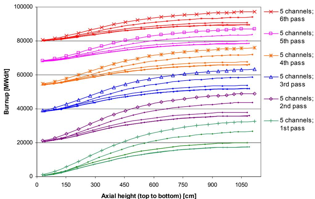
**Fig. 3** Accumulative burn-up of the fuel in five radial channels during six passes
