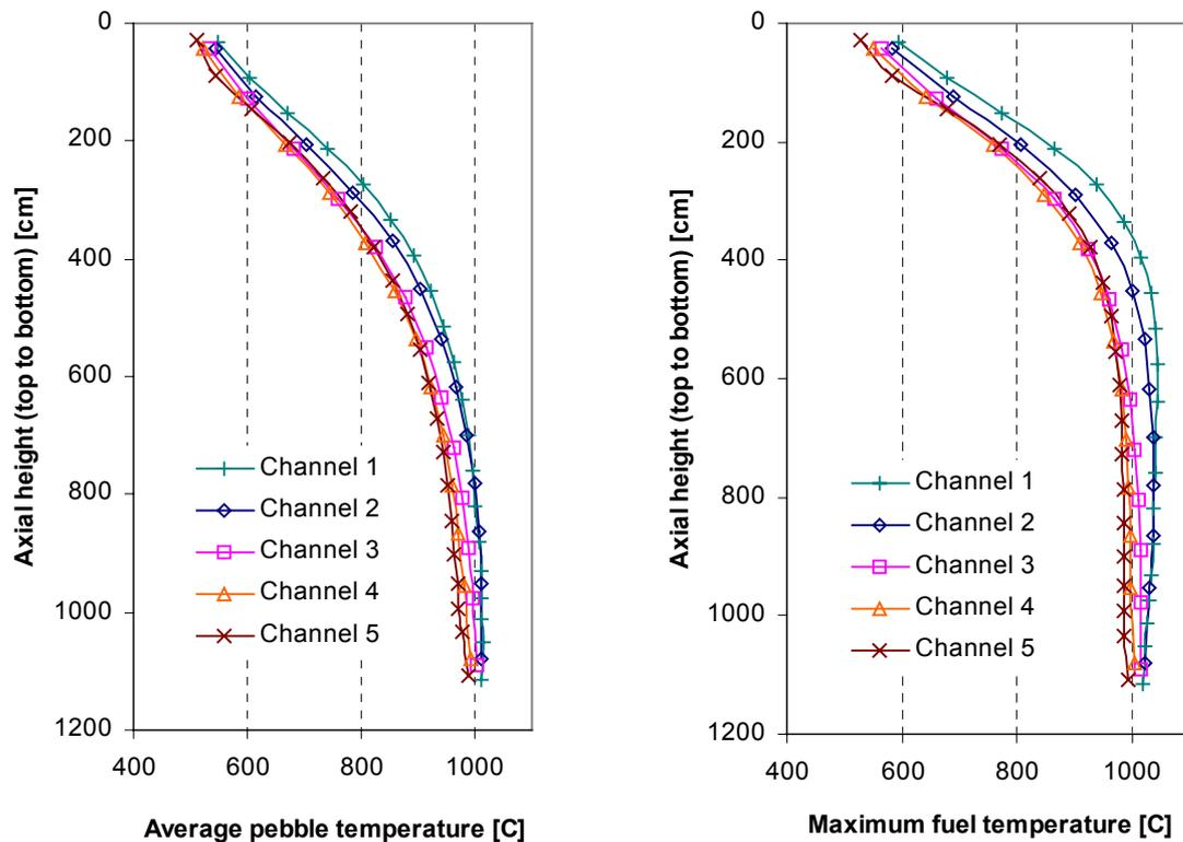
**Fig. 5** Fuel pebble average and maximum (centre) temperatures in °C for the pebble flow channels
