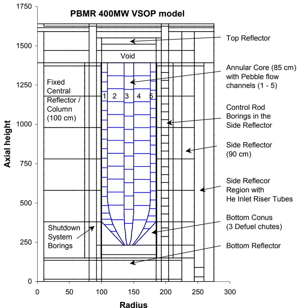
**Fig. 1** VSOP core geometrical model (R-Z cut) showing five flow channels in the annular core, the reflector regions and positions of reactivity control systems.
