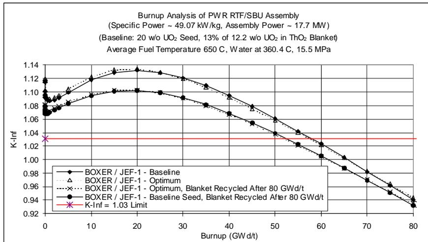
Fig. 2. BOXER Calculations of SBU Fuel Assembly Reactivity Variation with Burnup
