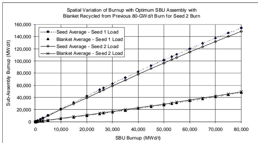
Fig. 3. Variation of Sub-Assembly Burnup Level with SBU Burnup
