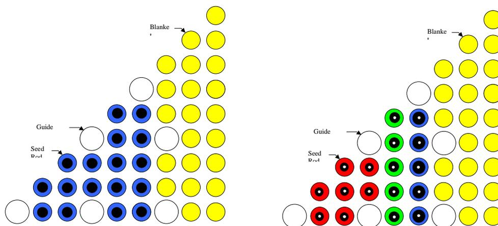
**Fig. 1.** Layout of Fuel Pins in 1/8<sup>th</sup> Baseline (left) and Optimized (right) SBU Designs
