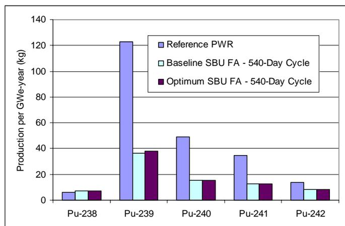
Figure 9: Plutonium Isotope Production per GWe-Year
