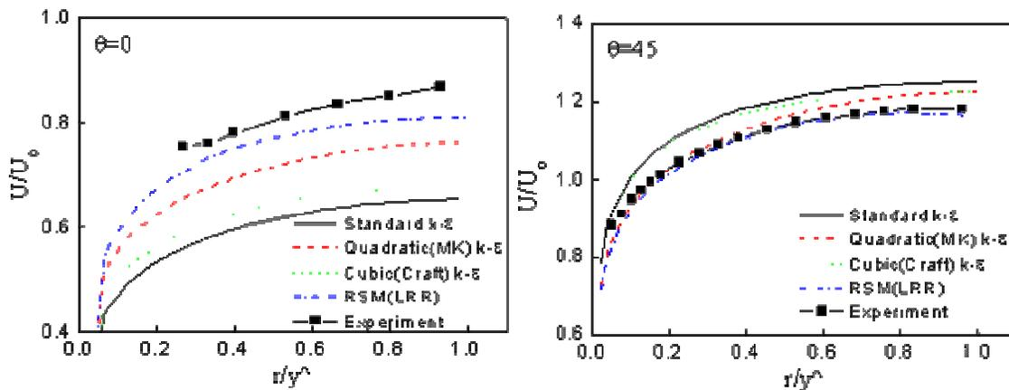
Figure 3. Mean Axial Velocity Distributions along the Gap ( $\theta=0^\circ$ ) and along the Diagonal ( $\theta=45^\circ$ ).
