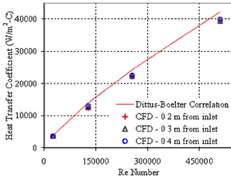
Figure 5. Heat Transfer Coefficient Comparisons with the Standard k- $\epsilon$  Model.
