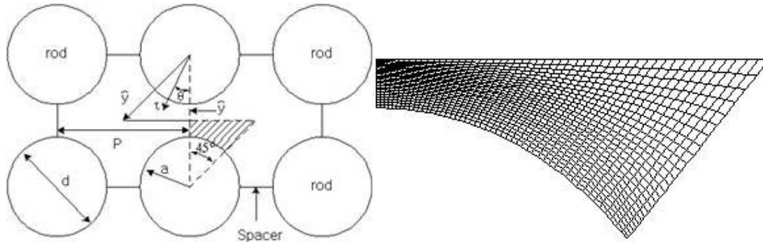
Figure 1. Schematic of Square Rod Bundle and Computational Grid of Octant Subchannel.
