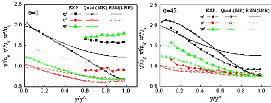
Figure 4. Comparisons of Turbulence Intensities along the Gap ( $\theta=0^\circ$ ) and the Diagonal ( $\theta=45^\circ$ ).
