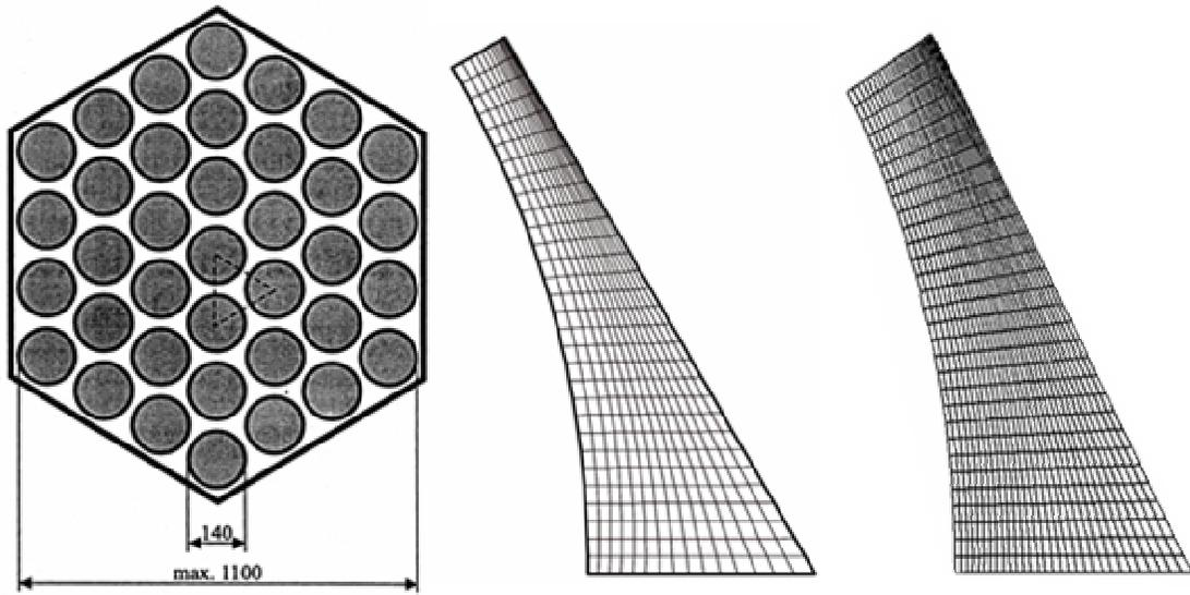
Figure 6. 37-rod heated bundle with triangular array, and the simulation grids for pitch-to-diameter ratio of 1.06 (middle) and 1.12 (right).
