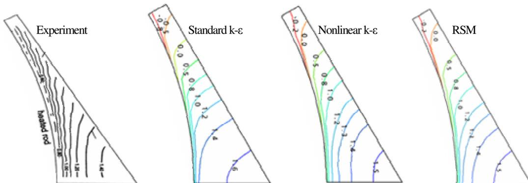
Figure 8. Time averaged temperature  $((T_{w,m}-T)/(T_{w,m}-T_b))$  distributions for  $P/D=1.06$ .
