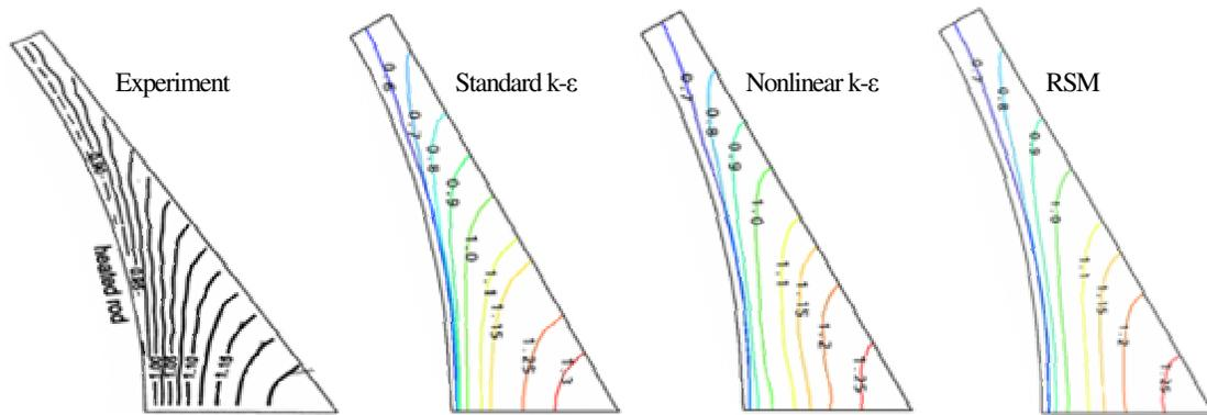
Figure 7. Distributions of mean velocity for  $P/D=1.06$ .
