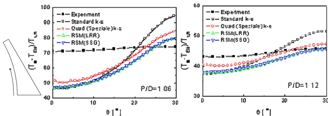
Figure 10. Distributions of dimensionless wall temperature.
