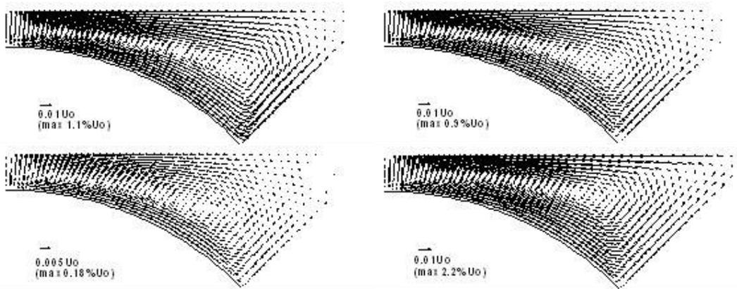
Figure 2. Turbulence-Driven Secondary Flow as Predicted by the Nonlinear Turbulence Models: (Clockwise from Top Left) Ref. 8, Ref. 9, Ref. 14, and Ref. 11.
