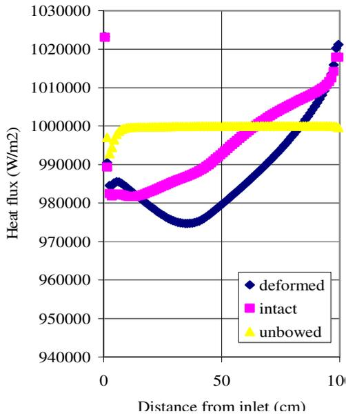
Fig. 12. Heat flux comparisons for the back surface (right surface of the pin in Fig.5).
