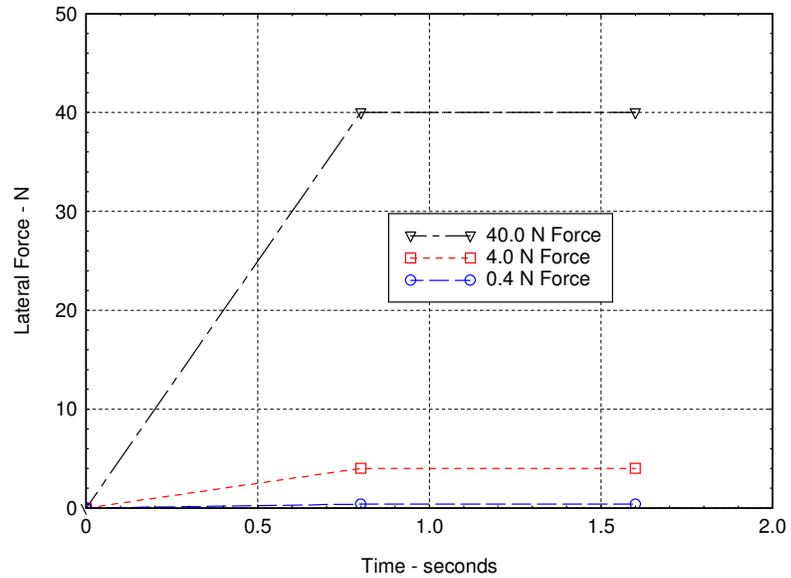
Fig. 2. Assumed Lateral Force Transient from Fluid Flow
