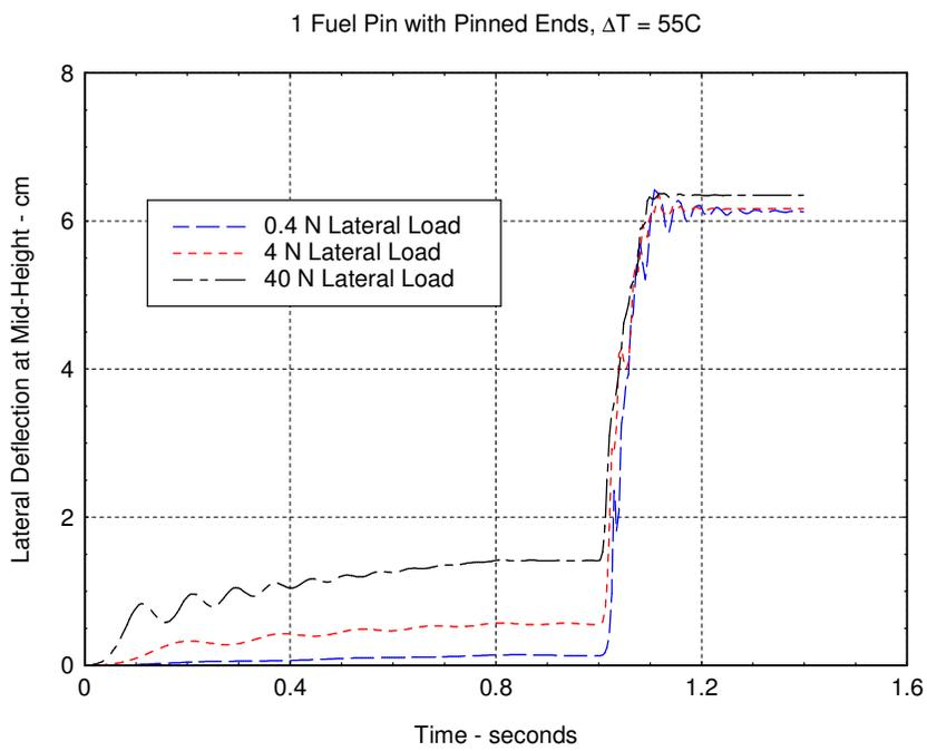
Fig. 4a. Lateral Deflection of Beam due to Lateral Force and Thermal Transient for 55C
