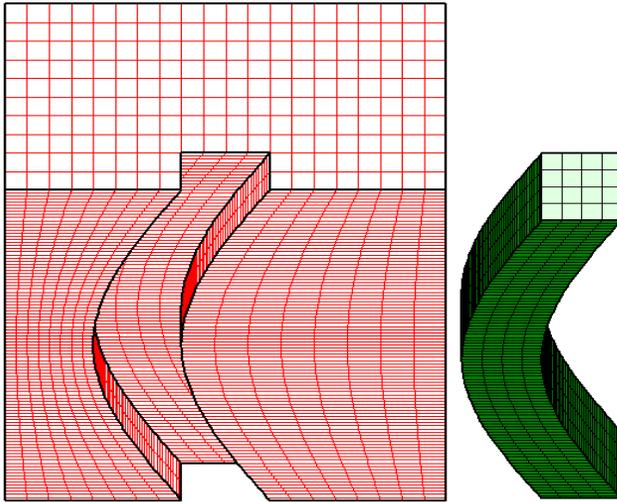
Fig. 10. Bowed configuration of square profile heated fuel pin (right) in the middle of a square profile coolant channel (only half shown on left).
