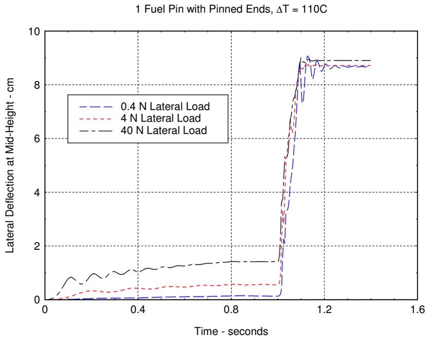
Fig. 4b. Lateral Deflection of Beam due to Lateral Force and Thermal Transient for 110C
