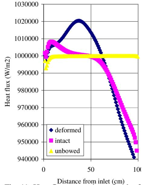
Fig. 11. Heat flux comparisons for the front surface (left surface of the pin in Fig.5).
