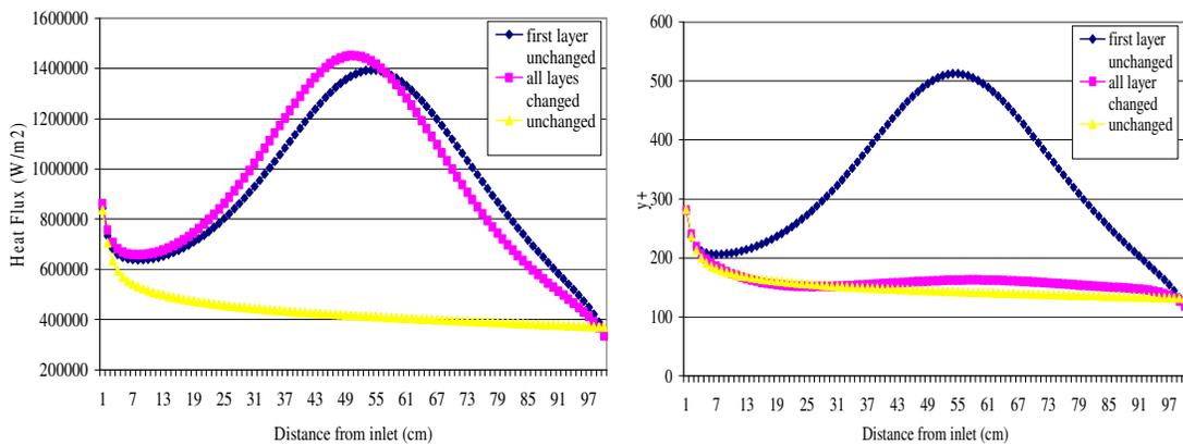
Fig. 9. Heat flux and  $y^+$  comparisons on the constant-temperature lower wall in Fig.8.
