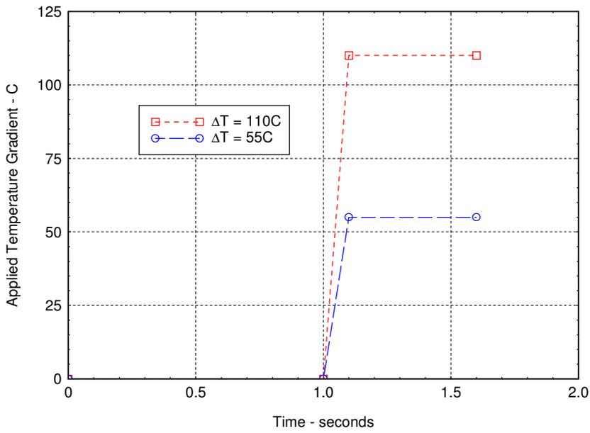
Fig. 3. Assumed Thermal Transient Acting in Beam
