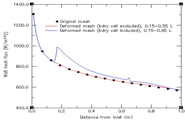
Fig. 7. Comparison of heat fluxes for the abruptly deformed mesh over 50% of the channel length to the case with the cell adjacent to the wall (boundary layer) kept the same size as the original mesh.
