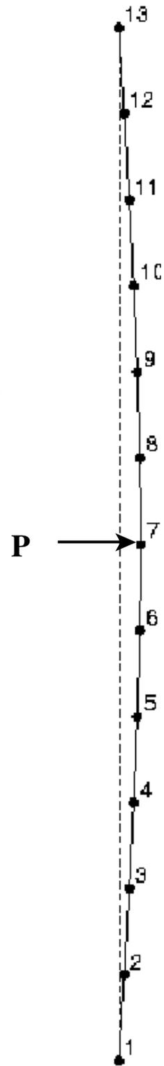
Fig. 5. Bowing of Beam due to Lateral Force and Thermal Transient
