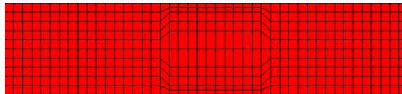
Fig. 6. Deformed mesh structure for 2-D flow between parallel plates.
