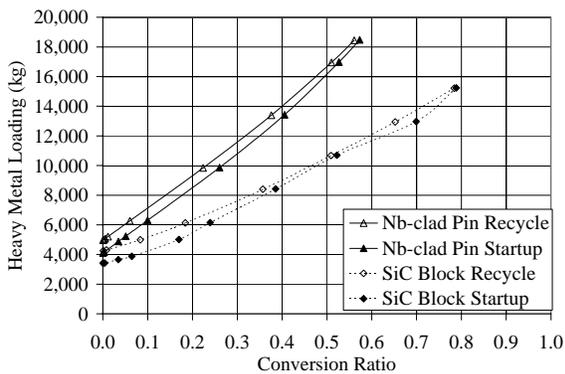
**Fig. 2.** BOEC Heavy Metal Loading
