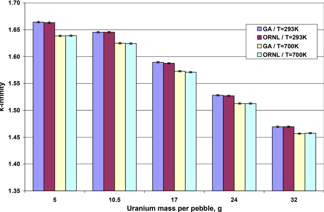
**Fig.9** k-infinity as a function of uranium mass per HTR UOX sphere
