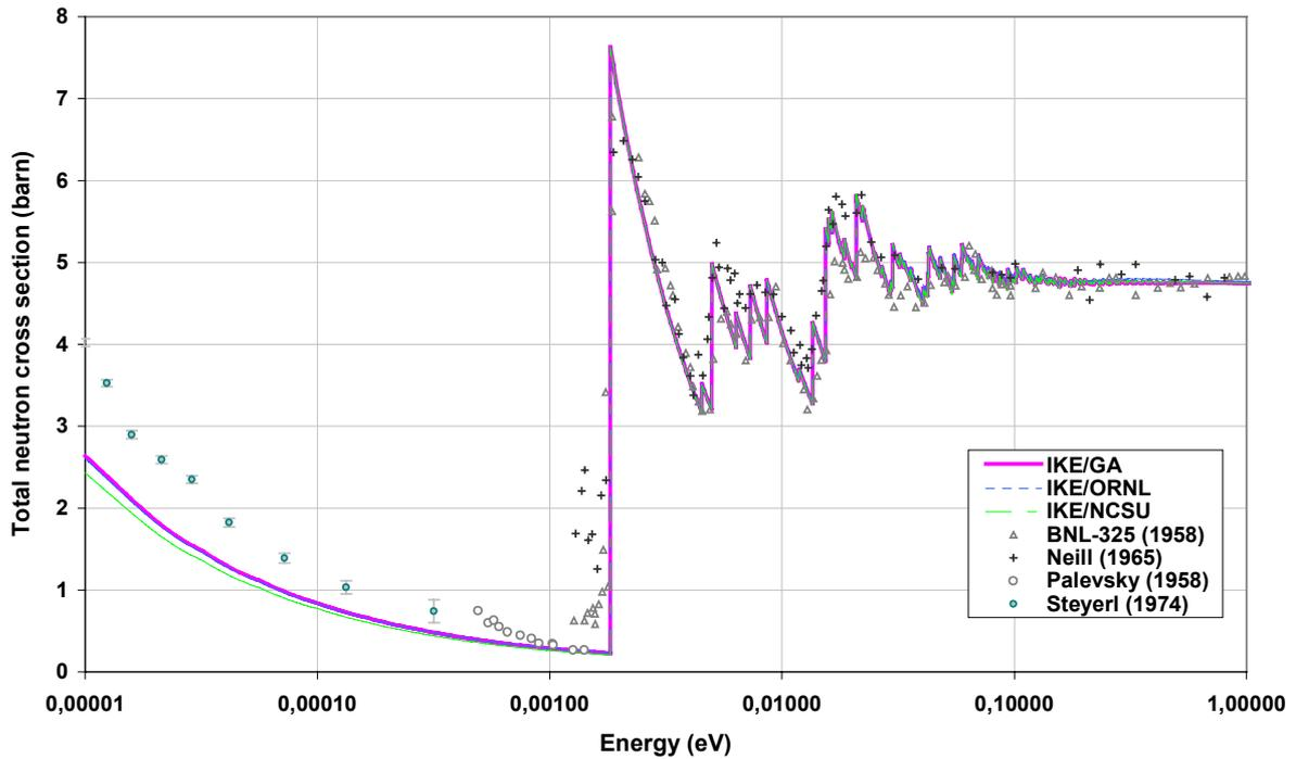
**Fig.7** Total neutron cross section of polycrystalline graphite for room temperature
