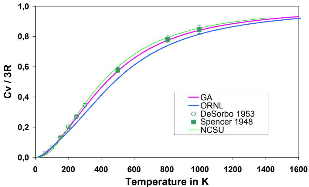
**Fig. 2** Specific heat for polycrystalline graphite
