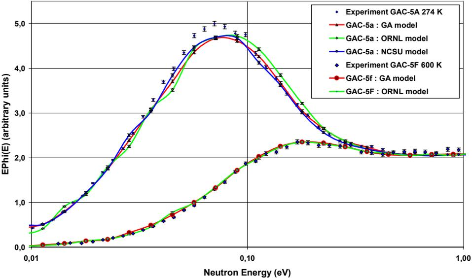
**Fig.8** Neutron spectra for the graphite Benchmark GAC-5A and GAC-5F
