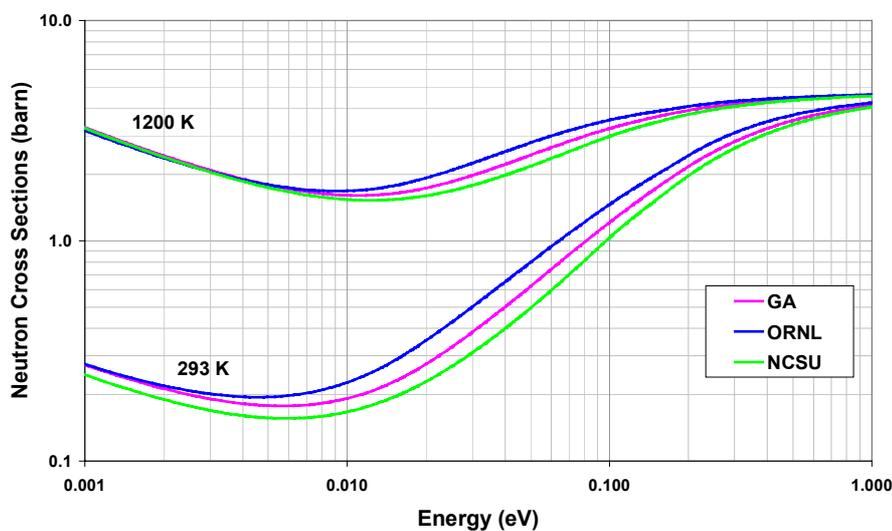
**Fig.6** Incoherent inelastic neutron cross sections for graphite
