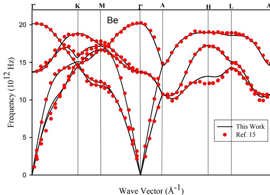
**Fig. 2.** The dispersion relations for beryllium based on a 96-atom supercell.
