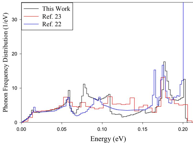
**Fig. 6.** The phonon frequency distribution for graphite.
