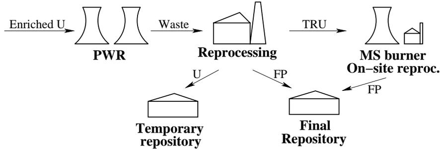
**Figure 1:** Simplified scheme of PWR - MS incinerator fuel cycle. Abbreviations: FP - fission products, TRU - transuranium isotopes, U - Uranium
