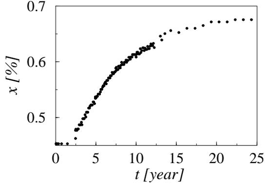
**Figure 3:** Evolution of the actinide molar concentration in carrier salt.
