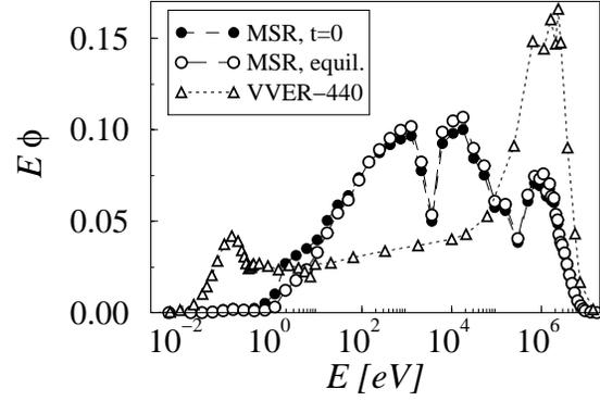
**Figure 4:** Average spectrum in the MS burner at the beginning of operation and at equilibrium, compared to the spectrum of a VVER-440 assembly.
