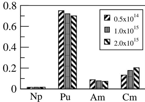
**Figure 5:** Fractions of the main transuranium elements at equilibrium as a function of the neutron flux
