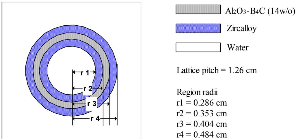
**Fig.1 B<sub>4</sub>C in alumina pin cell**
