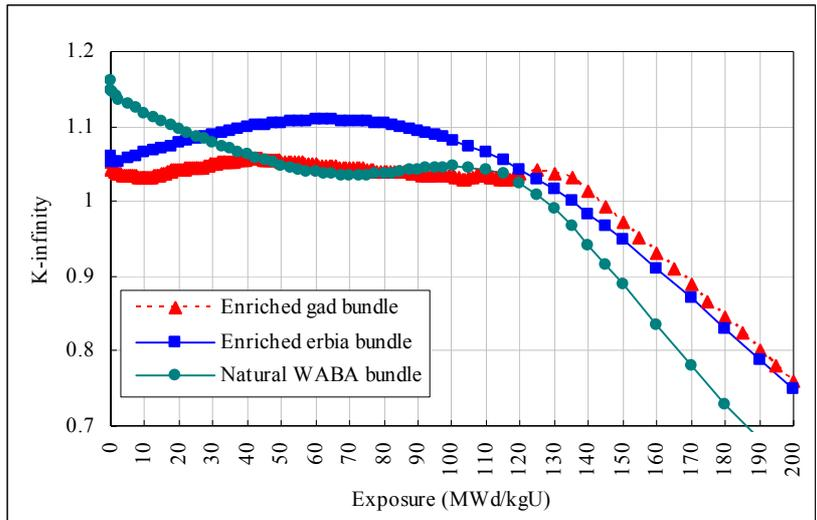
**Fig. 2 Comparison of K-inf at 40% void**
