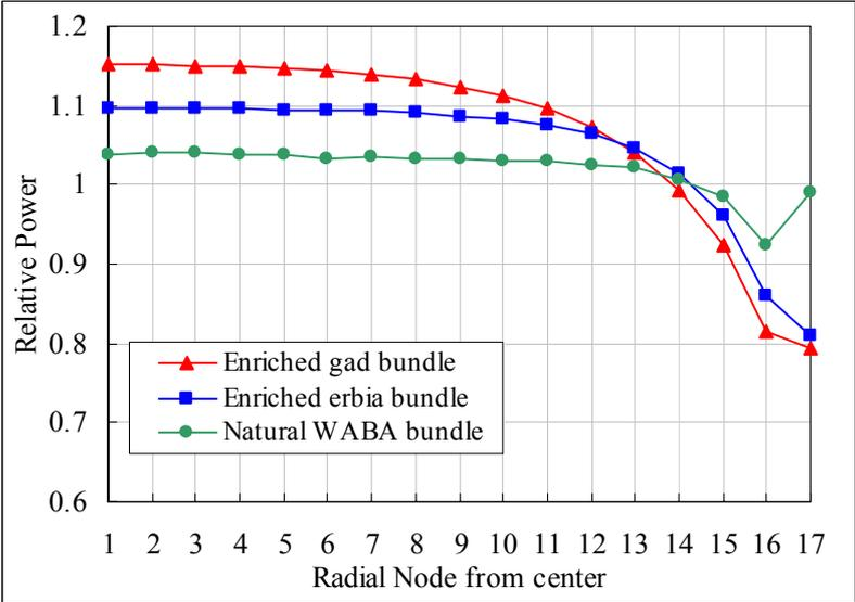
**Fig. 5 Comparison of Haling radial power distributions**
