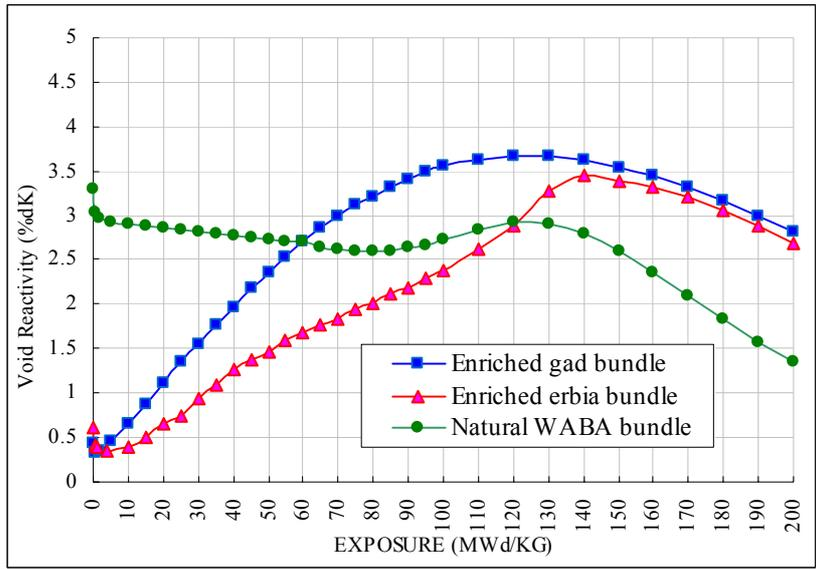
**Fig.4 Comparison of Void Reactivity (40 to 0% void)**
