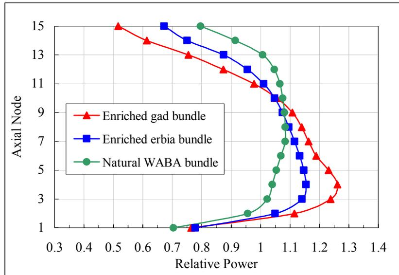
Fig. 6 Comparison of Haling axial power distributions
