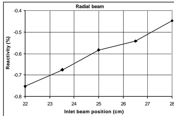
**Fig.6** Reactivity changes as a function of the inlet beam position for radial beams.
