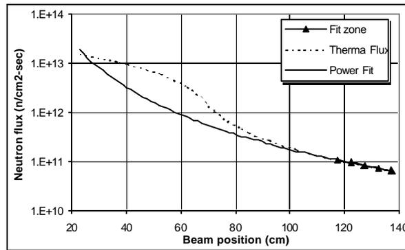
**Fig.8** Power law fit over the thermal flux at the beam's end.
