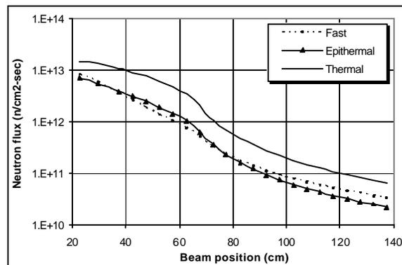
**Fig.3** Typical neutron flux distribution along the radial beam.
