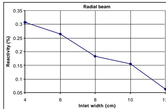
**Fig.14** Reactivity changes decreasing the inlet width of R2 case.
