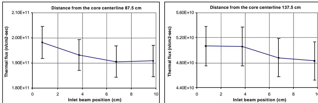
**Fig.10** Thermal flux variation vs. inlet beam position for tangential beams.
