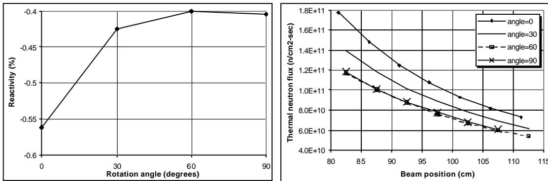
**Fig.17** Reactivity variation and thermal flux distribution for the beams in different angular positions. An angle of zero degree corresponds to the tangential beam.
