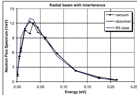
**Fig.21** Flux spectrums with and without device interference.
