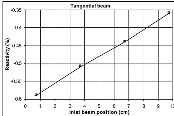
**Fig.11** Reactivity changes as a function of the inlet beam position for tangential beams.
