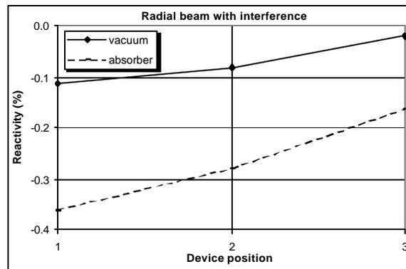
**Fig.19** Reactivity variation for the vacuum and absorber cylinders at three different locations.
