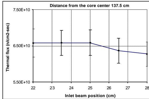
**Fig.5** Thermal flux variation vs. inlet beam position for radial beams.
