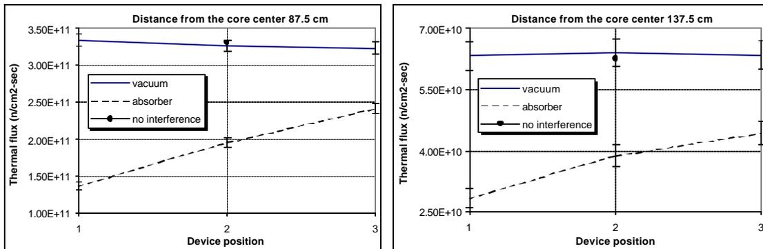
**Fig.20** Thermal flux distribution along the beam.
