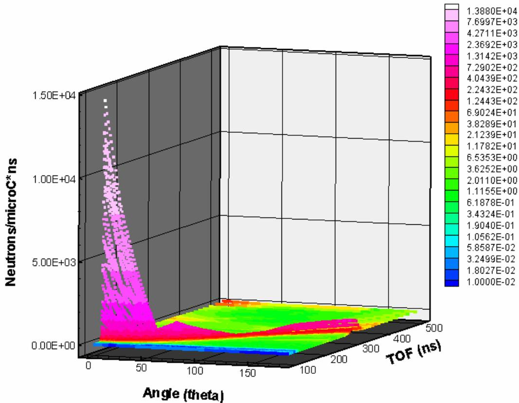
**Fig9** Complete Corrected D(d,n) Source Distribution for incoming 5 MeV deuterons
