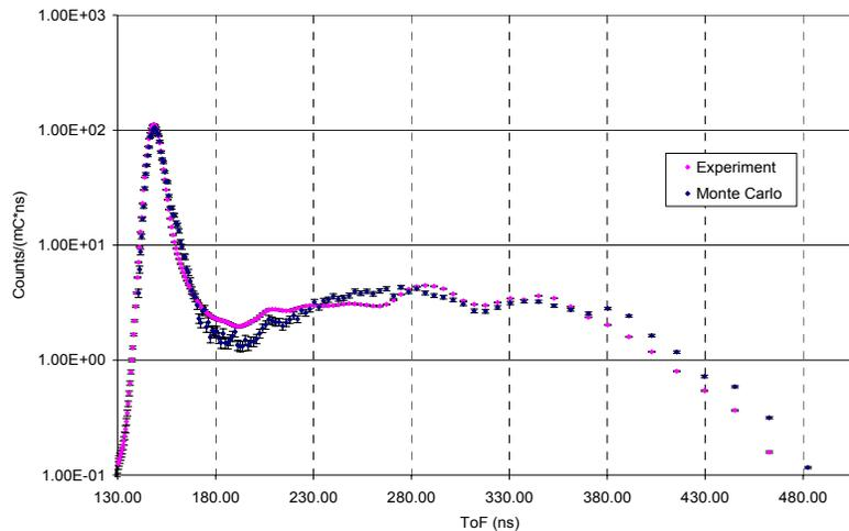
**Fig. 11** Comparison of the D(d,n) Monte Carlo Calculations for 3 MeV incident deuterons and Experimental Data for the 0 Degree Angle
