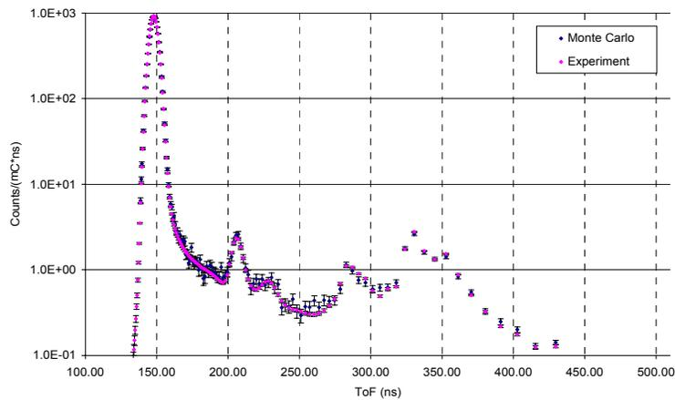
**Fig.10** Comparison of the D(d,n) Monte Carlo Source Calculations for incident deuterons of 3 MeV and Experimental Data for the 0 Degree Angle
