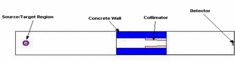
**Fig. 2** Y-Z Schematic of MCNP Model Utilized
