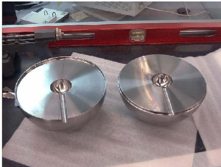
**Fig.7** 8cm Thick Iron Shell, Unassembled
