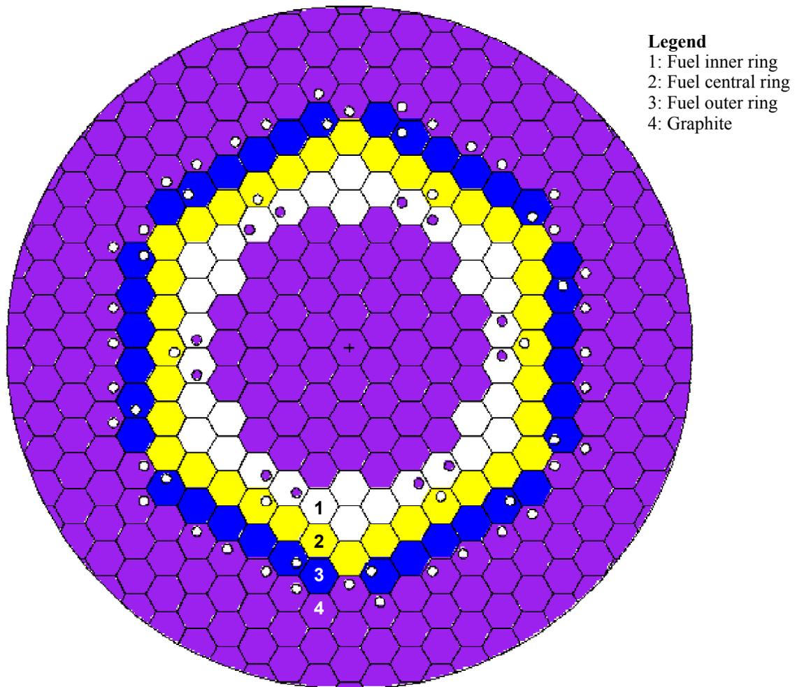
**Figure 1:** GT-MHR core design. The inner ring of fuel (white) contains 12 startup control rods, the central (yellow) and outer ring (blue) respectively do 6 and 12 shutdown control rods, the outer graphite reflector ring does 36 operational control rods.
