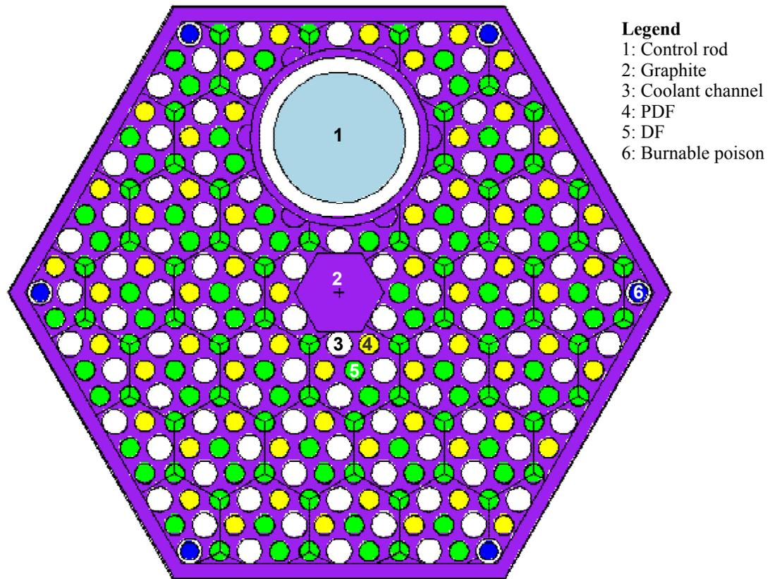
**Figure 2:** Hexagonal fuel block. The graphite matrix contains 95 coolant channels (white), 124 DF pins (green), 62 DF pins (yellow), 6 burnable poison pins (blue) and 1 (startup/shutdown) control rod (light blue).
