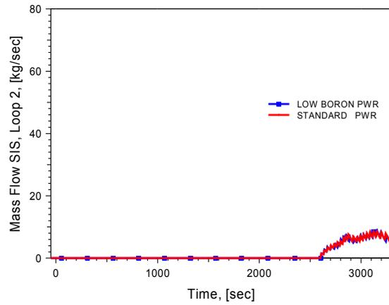
**Figure 7:** Mass flow in cold leg 2
