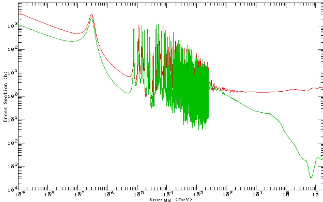
The spectral softening effect resulting from the use of BeO diluent is also beneficial from a void reactivity standpoint. Reactivity in this core is driven primarily by Pu-239, which accounts for ~65-70% of fissions throughout core life. It can be shown that:
