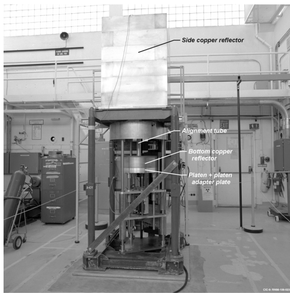
Figure 1. The Zeus Assembly Mounted on the Comet Machine.
