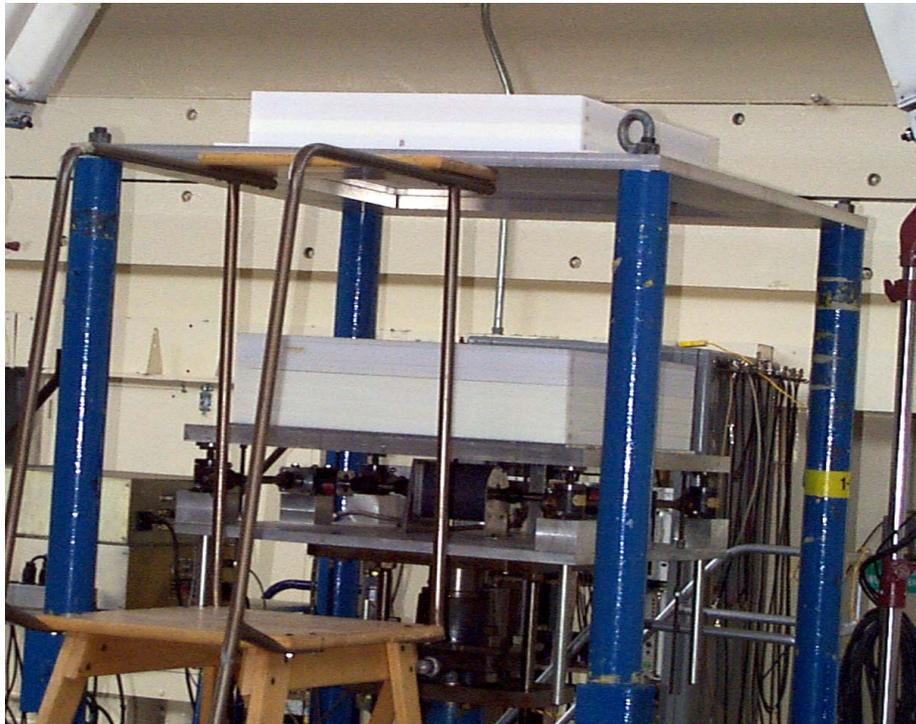
The experiments consisted of placing HEU foils interspersed with the waste materials ( $\text{SiO}_2$  plates, Al plates or Fe plates) in a short and fat column stack. The uranium foils were moderated and reflected by polyethylene square plates. A unit consisted of one polyethylene plate with a recess in its top side that contained the four waste material plates being examined and four HEU foils on top of the waste material plates.
